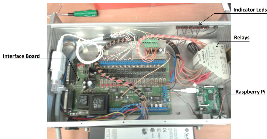
Figure 3: Inside components of the new control unit
