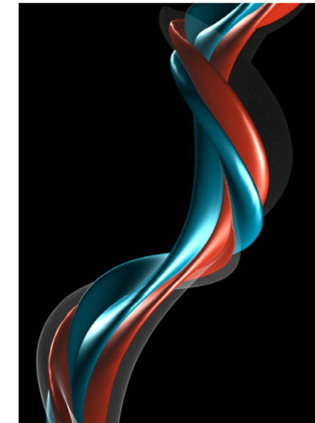
Helical optical shock in generalised superradiance. Superradiant radiated electric field recorded in a virtual detector as a function of time (vertical direction) and transverse position. Blue/red refers to negative/positive electric field values. The optical shock forms a helix.
