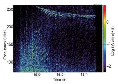
Spectrogram of density perturbations from O-mode interferometry on JET discharge #66203, with tornado modes visible around 225-250 kHz while AC sweep the frequency range 100-225 kHz.
