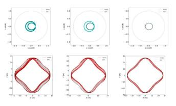
Orbits of fast particles in quasi-helically symmetric stellarators [2].
