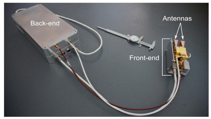
Microwave interferometer prototype.
