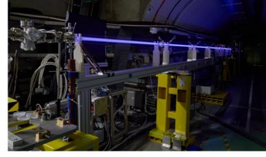
Discharge Plasma Source mounted in the AWAKE facility at CERN in April 2023, producing a 10 m long argon plasma.
