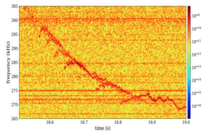
Spectrogram of MHD activity from interferometry diagnostic in the TAE range of frequencies for JET pulse #69247.
