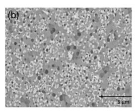
(b) high magnification of the microstructure of the consolidated (CrTaW)\_{\infty}Fe\_{z}Ti\_{z} sample.
