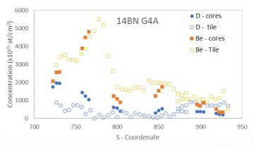
2300keV in Tile: 14BN G4A Comparison of fuel retention on the cores and full tile.
