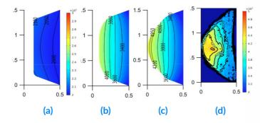
The cathode tip shape and the temperature distribution in the tip. (a)-(c): Modelling, t=295 ms (a), 331 ms (b), 1 s (c). (d): Experiment, stable mode. The spatial dimensions are in millimetres and the temperature bars in kelvin. Temperature bars for frames (b) and (c) are the same as for frame (d).
