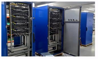
The first assembled cubicles with electronics of the ITER magnetics diagnostic, of 17 to be delivered. In total, 1699 integrators will be installed in the 17 cubicles (and there are 340 spares that will be delivered separately). There are 24 integrator variants for different magnetics-sensor types.
