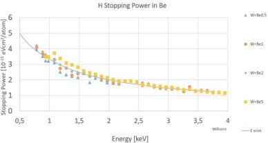
Stopping power of H ions in Be as function of incident energy.
