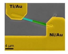
SEM image of a core-shell GaN nanowire device.
