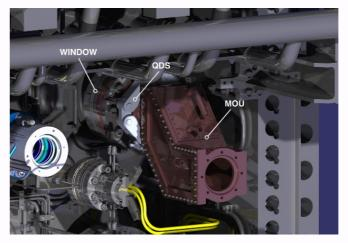
CTS launcher's Matching Optics Unit (MOU), which contains a two-mirror setup that provides support, cooling, and maintains the vacuum boundary of the transmission line. The Quick Disconnection System is also shown, facilitating the easy and rapid detachment of the MOU from the window.
