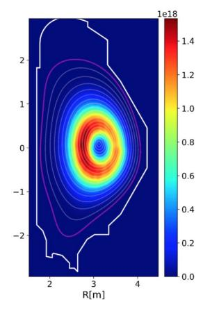
Spatial distribution of energetic particles from the negative beam source as calculated by ASCOT.
