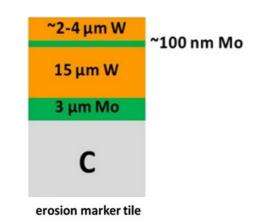
Erosion marker tile as-deposited on a carbon fibre composite.
