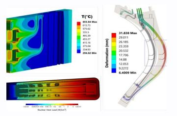
Waveguide deformation due to thermal loads - Due to the harsh radiation environment of DEMO, reflectometry waveguides will be subjected to radial deformation during operation. What is the impact on the measurements?
