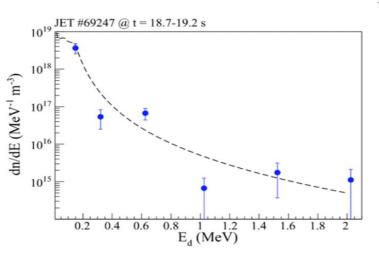
Distribution in energy of the energetic D population as deduced from the spectrum of D-D produced neutrons measured by TOFOR in pulse #69247 (blue dots) compared to prediction from PION code (black dashed line, bottom).
