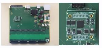
(Left) ATCA-MIMO-ISOL-V2 data acquisition and processing board developed for W7-X Stellarator CODAC; (right) the IPMC module installed on the ATCA ATCA-MIMO-ISOL-V2.
