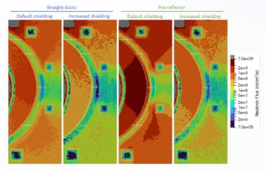
Radiation loads in the magnets - Introducing diagnostics in the DEMO equatorial ports increases the fluxes in the toroidal and poloidal field coils. Different design and shielding configurations have been tested for the X-ray diagnostic, to ensure that the flux and load limits are not exceeded.
