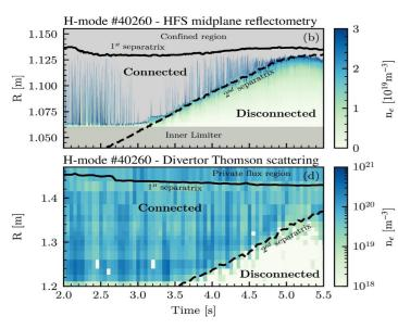
HFS SOL density contour as a function of time and major radius at the HFS midplane using O-mode reflectometry and at the divertor using Thomson scattering from anH-mode shape scan.
