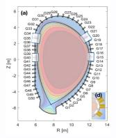
(a) The DEMO PPR concept includes multiple reflectometry lines of sight (LOS) distributed poloidally around the machine.
