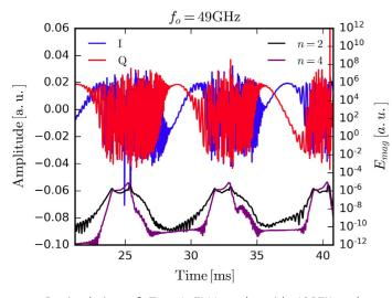
3D simulation of Type-I ELM cycle with JOREK code and corresponding 2D synthetic reflectometry measurements with REFMUL code. 24
