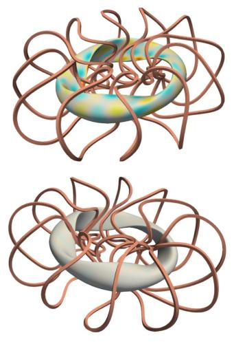
The simplification of coils of a 3 field period quasi-axisymmetric device with a lower coil ripple [3].
