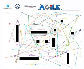
The path planning algorithm is designed for transportation trolleys in dense and confined scenarios, including maintenance operations in nuclear facilities. It is particularly suited for transportation missions between reactor and hot cell buildings.
