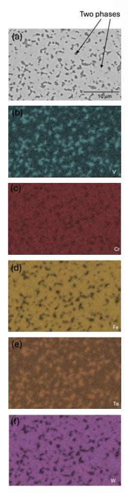
EDS map of the (a) consolidated CrFeTaVW for (b) V-K $\alpha$ , (c) Cr-K $\alpha$ , (d) Fe-K $\alpha$ , (e) T-L $\alpha$  and (f) W-L $\alpha$  lines.
