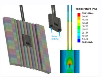
Laboratory measurements showed excellent agreement with REFMUL3 simulations, validating the accuracy of the code. (Right) thermal analysis of a cooled bistatic antenna block embedded in the current FW standard module configuration during continued DTT operation.
