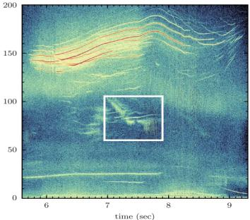
Magnetic-coil power spectra for JET pulse #90199: ICRH-driven Alfvénic activity, with TAEs around 150 kHz and lower frequency AEs in the range between 60 and 100 kHz (inside the white box), evidencing the bursty frequency bands surrounding sharp frequency lines.
