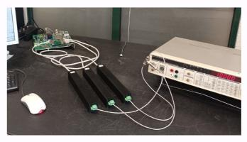
ENOB test rig with the production samples being tested.
