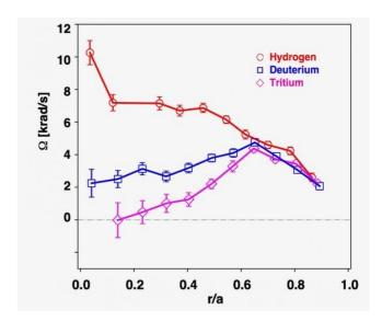
H, D and T toroidal angular frequency profiles with the same density <Ne> ~ 2.35 × 10<sup>19</sup> m<sup>-3</sup>, for plasmas with Ip = 2.3 MA, BT = 2.7 T.
