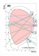
(b) A new diagnostic approach is being developed for the ramp-up phase, where the PPR hardware will function as an interferometer (1), refractometer (2), intensity refractometer (3), or in standard reflectometer mode (4).
