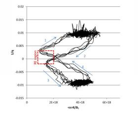
Murakami-Hugill characteristics of ISTTOK alternating discharges revealing runaway populations contributions for the plasma current (elbows in points A and B).
