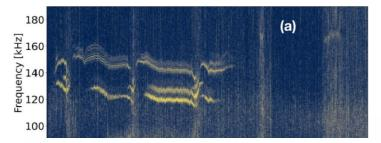
Spectrograms in the TAE range of frequencies corresponding to ASDEX-UPGRADE discharge #38012 (no ECCD).
