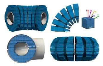
Design of ISTELL - a non-axisymmetric version of ISTTOK using permanent magnets [1].
