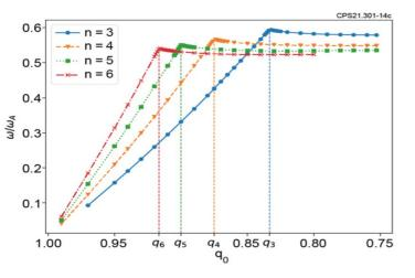
Simulated evolution of the frequency with the on-axis safety factor value qO for the toroidal mode numbers n = 3, 4, 5, and 6.
