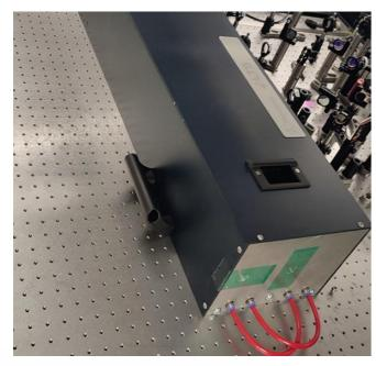
Multipass cell system installed at L2I.
