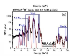
PIXE (c) spectra with corresponding fit lines achieved from the elemental analysis.
