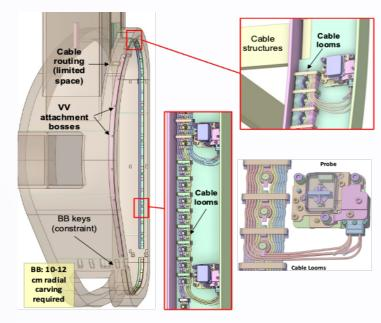
'Magnetics strip' - Will the magnetic sensors survive long-term neutron irradiation? An innovative concept has been proposed for the integration of magnetic sensors in DEMO, compatible with Remote Handling.
