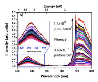
Lonoluminescence evolution of a single crystal of Cr-doped Ga<sup>2</sup>O<sup>3</sup> as a function of protons irradiation fluence;
