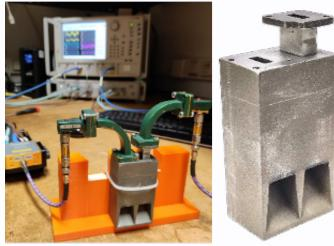
Installed in the microwave laboratory for performance analysis (centre). DMSL printed bistatic antenna prototype (left).
