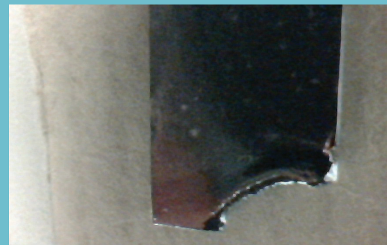
Eroded tungsten sample during an ISTTOK AC discharge.
