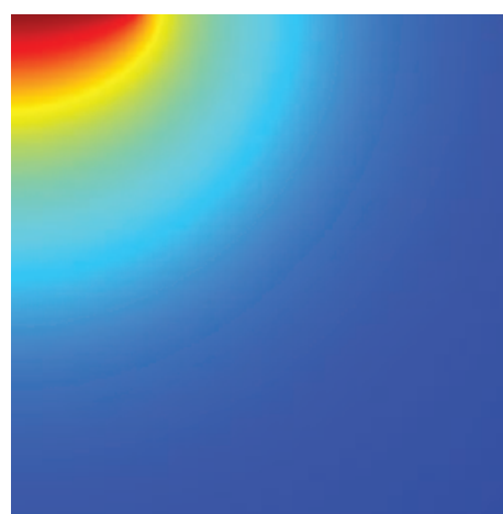
Axially symmetric spot on a Cu cathode of vacuum arc. Arc current 47 A.
