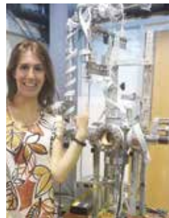
Wettability studies on ISTTOK Experimental setup built to investigate high purity liquid gallium wetting processes on stainless steel samples.
