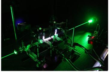
motivated by the environmental problems of climate change and the production of "green fuels". Low-temperature plasmas are one of the best ways for decomposing this gas – the separation of the molecule into oxygen and carbon monoxide – a process that happens either by colliding with electrons or by transferring energy to different states of excitation.
