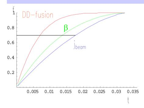
fractional contribution f of fast particles to DD-fusion,  $\beta$ , and beam current during first t seconds of their slowing down history
