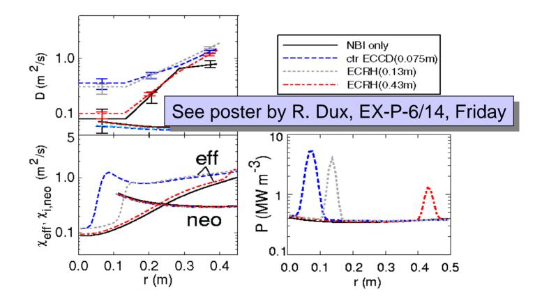
Effect of central heating on density peaking (neoclassical inward pinch) and on anomalous particle transport
