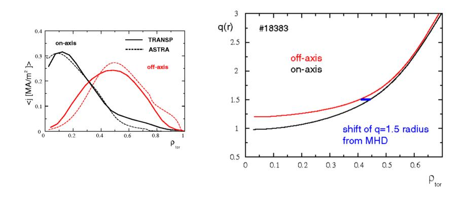
Current profile modification as predicted by TRANSP (MSE) – thanks to PPPL for support and consistent with shift MHD (shift of  $r_{3/2}$ )
