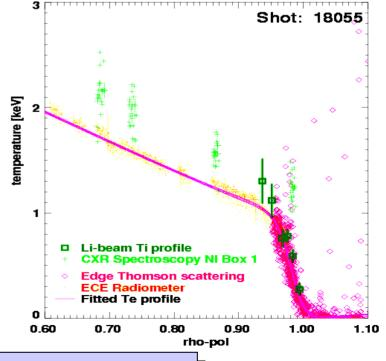
d log T<sub>e</sub>/d log n<sub>e</sub>~ 2 confirmed
