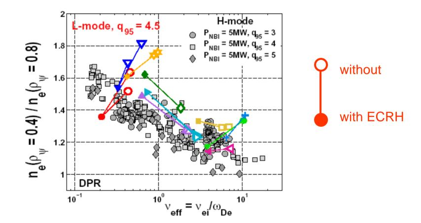
Reaction of density profiles and corresponding time scales again consistent with quasi-linear ITG/TEM model
