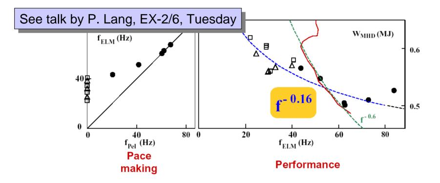
• only minor confinement degradation with increased ELM frequency compared to, e.g., gas puffing (pedestal temperature reduced!)
