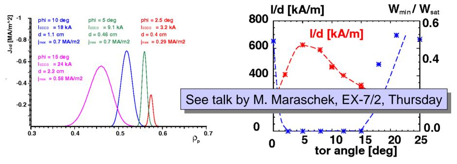
optimum launching angle: 5°, corresponds to 1 cm deposition width
