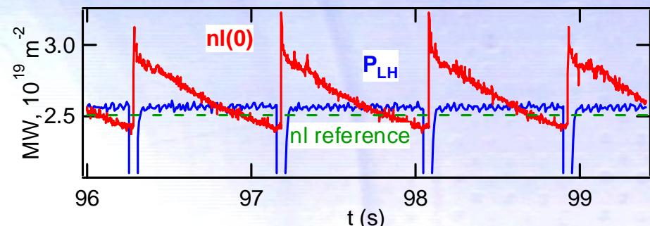
LH power notching allows penetration of 155 pellets
