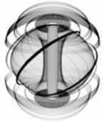
Plasma ring formation and merging clearly seen on centre column magnetic array
