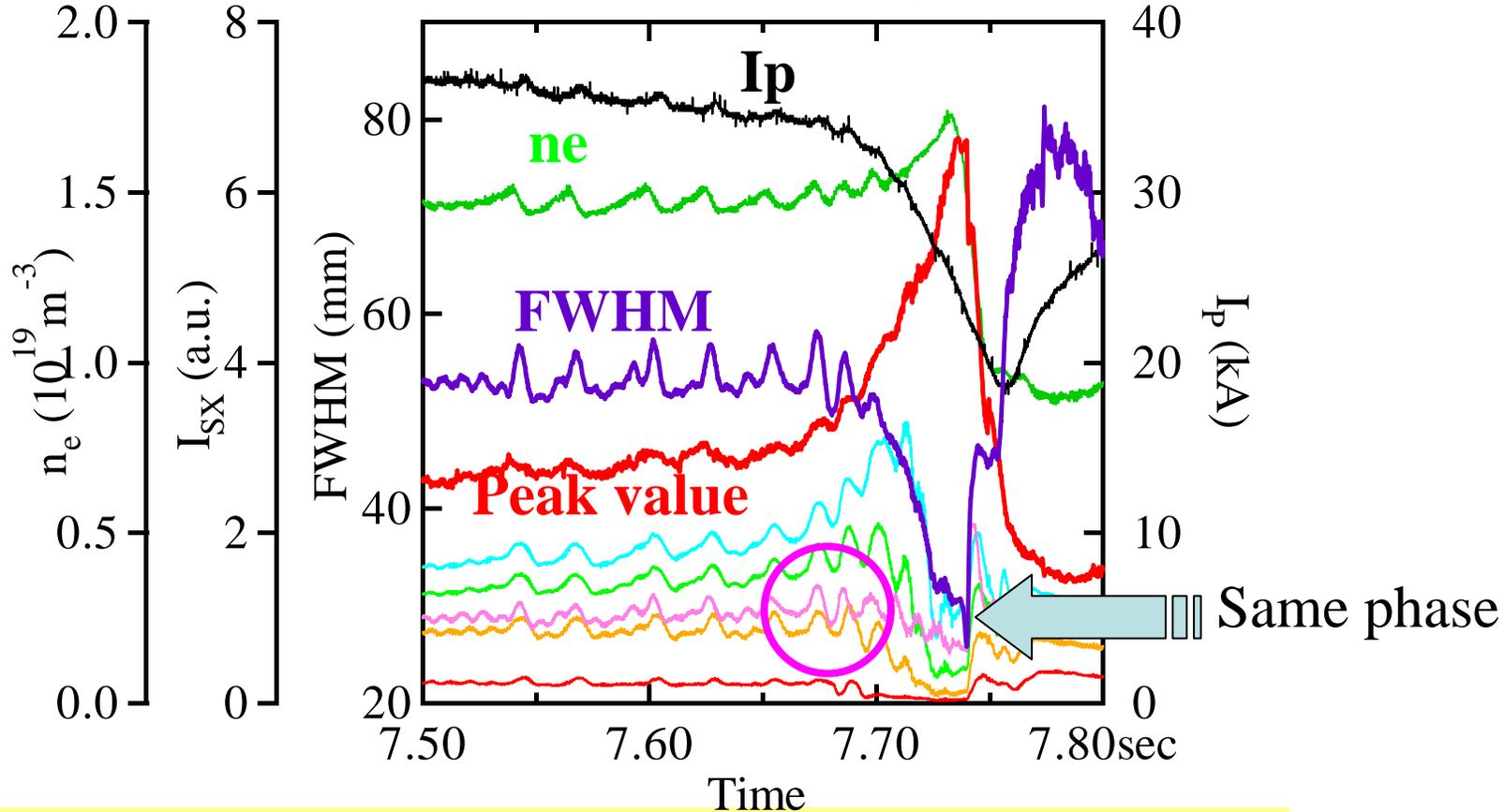
◆  $m=0$  type oscillations found on  $n_e/SX$  signals before the crash, indicating radial oscillation of ITB foot.
