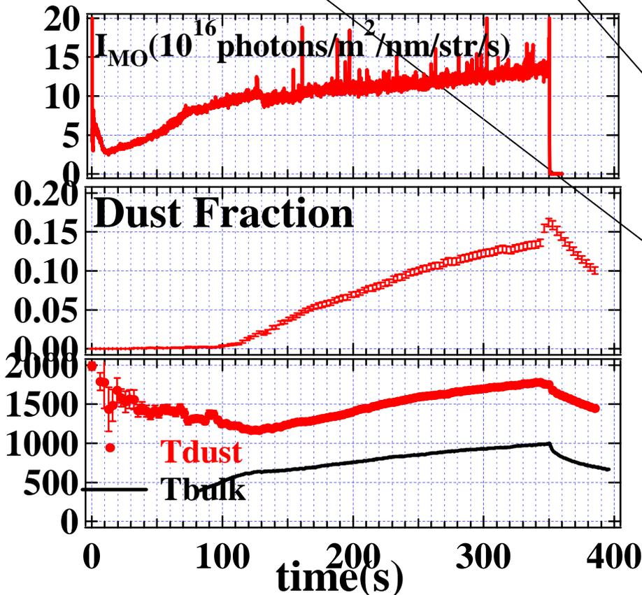
Three measurements in connection with dust deposition on different PFCs.
