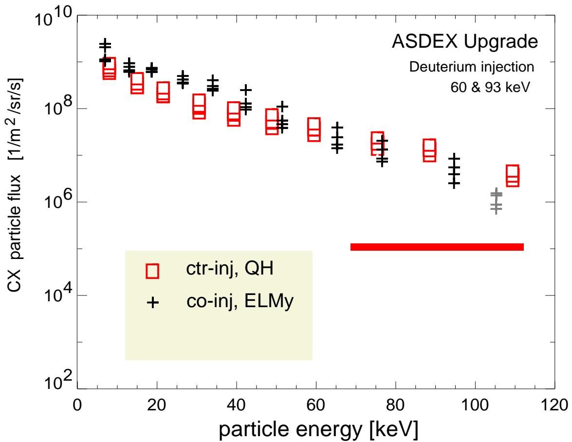
**Counter-NBI:** Higher yield than in with co-injection around beam energies (60 and 93 keV) despite lower density of thermal neutrals
