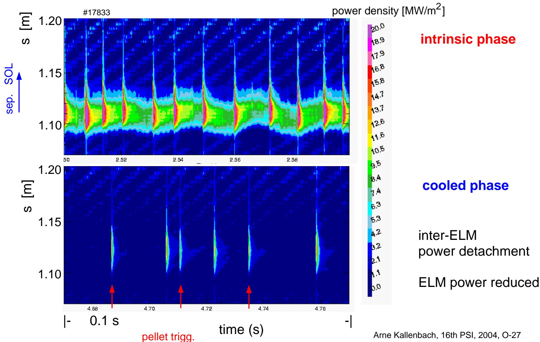
IR thermography viewing outer divertor target power load:
