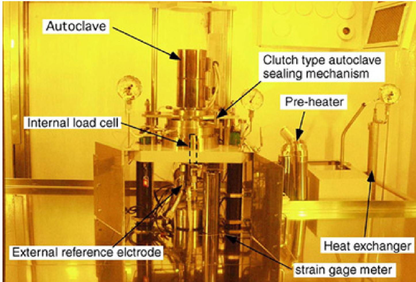
Slow Strain Rate Tensile test machine equipped in a hot Cell. SSRT tests were performed at 280°C after Irradiation to 2 dpa.
