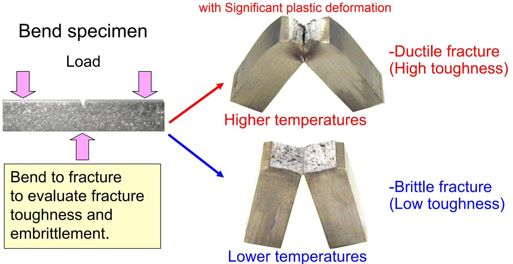
At low temperatures, steel fractures very easily;
