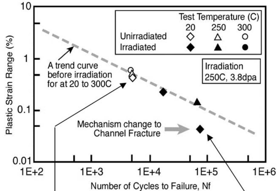
Small irradiation effect on fatigue property may allow application of current Design methodology.
