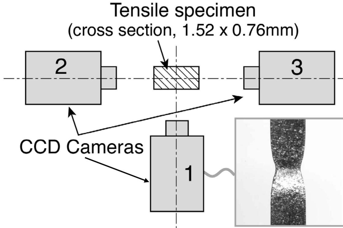
To measure the strain distribution in the neck at the gage section of the specimen, images of the specimens have been recorded continuously during the tensile test. Tensile direction is perpendicular to the sheet. 16
