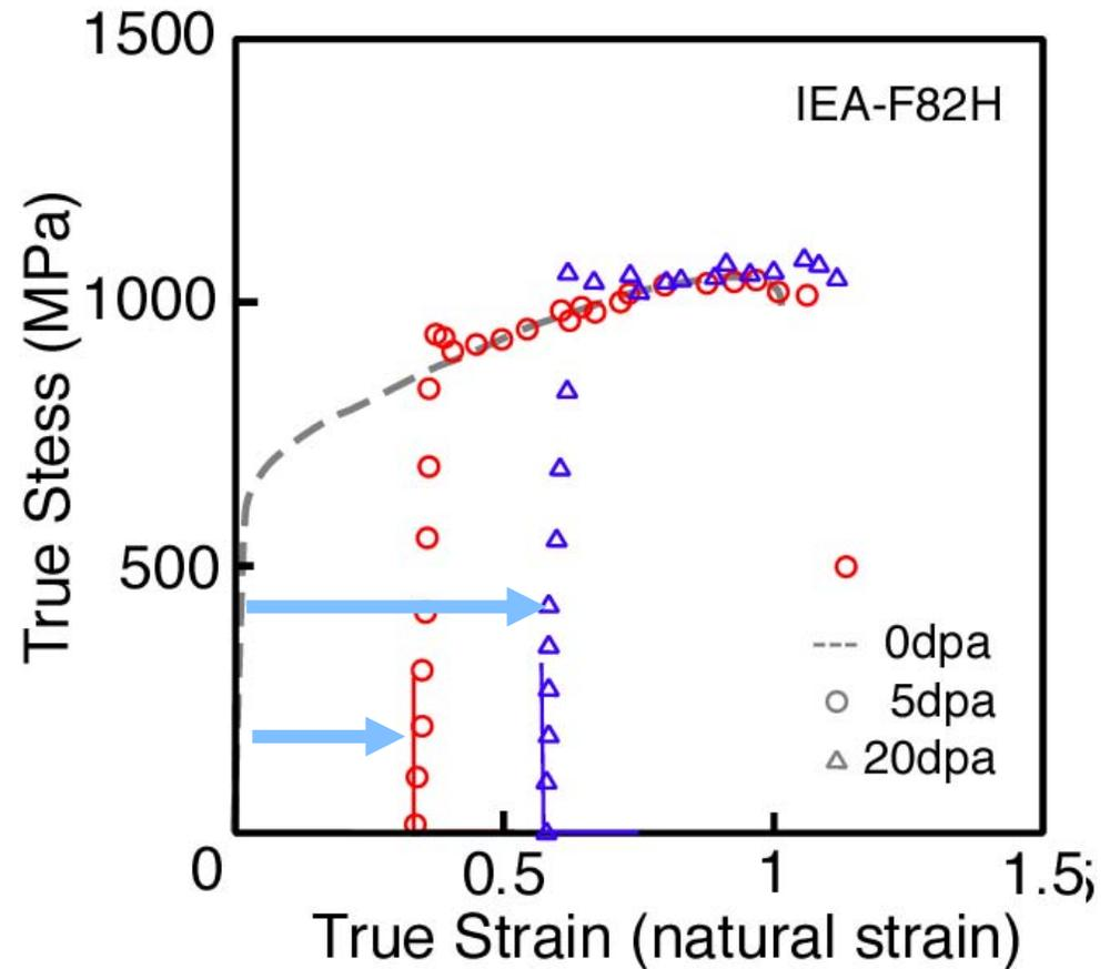
Results suggest that cold worked hardened material may be used to estimate the deformation and fracture of the irradiated component under monotonic loading. <sup>17</sup>
