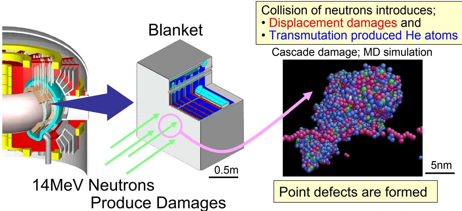
RAF/Ms FW will be damaged to 150dpa (+1500appmHe) by fusion neutrons from plasma at temperatures ranging from about 300C to 500C or even higher.
