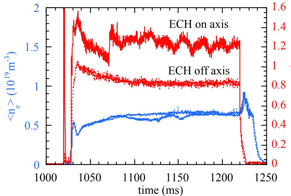
For the same density and magnetic configuration (close to  $n/m=3/2$ ), the eITB appears in the high absorbed power case.
