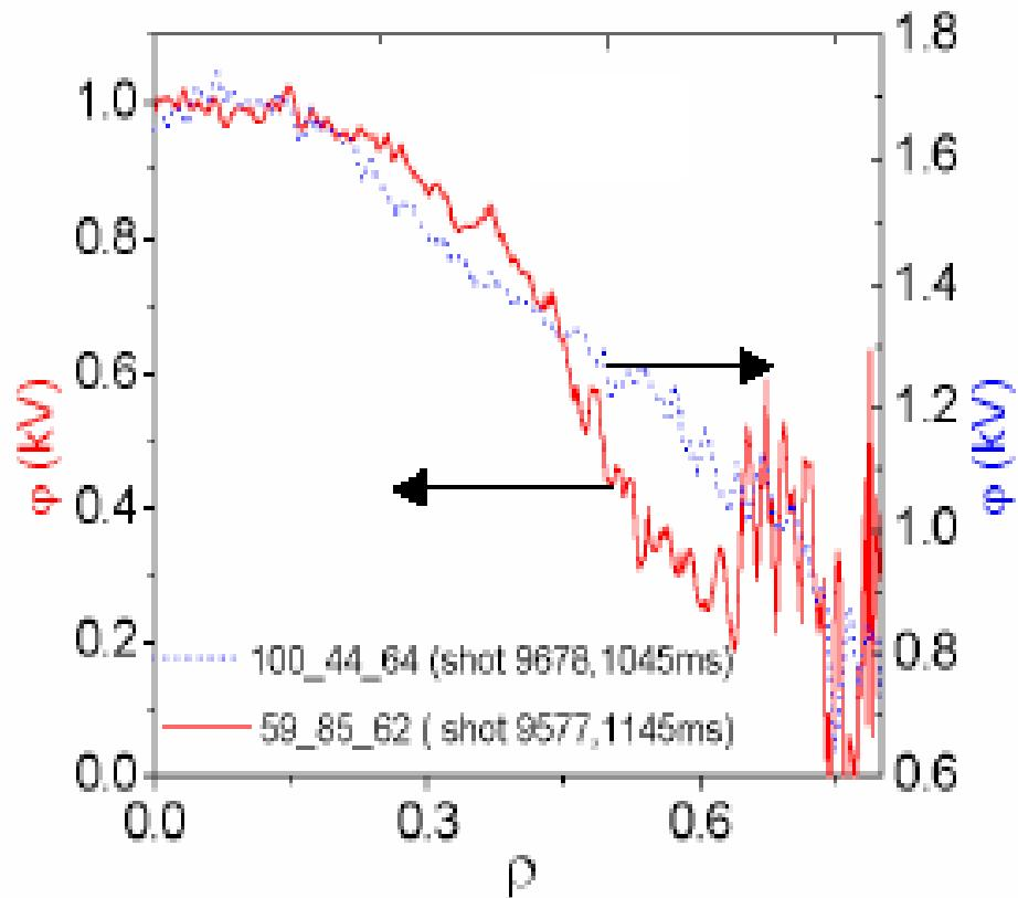
*Electric potential profiles in presence of  $n=4, m=2$  resonance in the plasma periphery (red) and without low order resonances (blue).*
