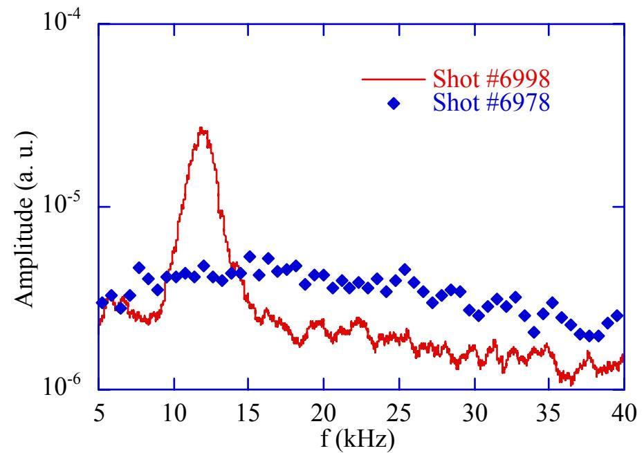
Coherent mode detected by Mirnov coils in the case with eITB.
