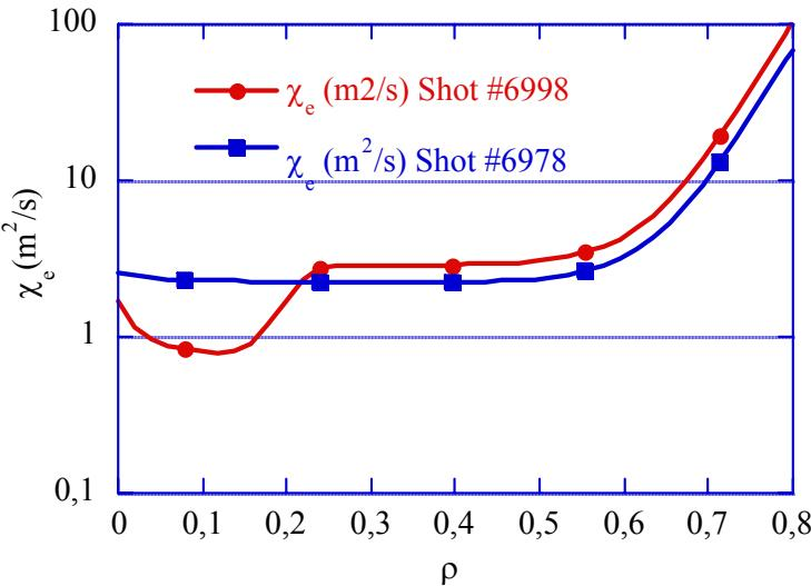
Heat conductivity with eITB is reduced in a factor two in plasma core.
