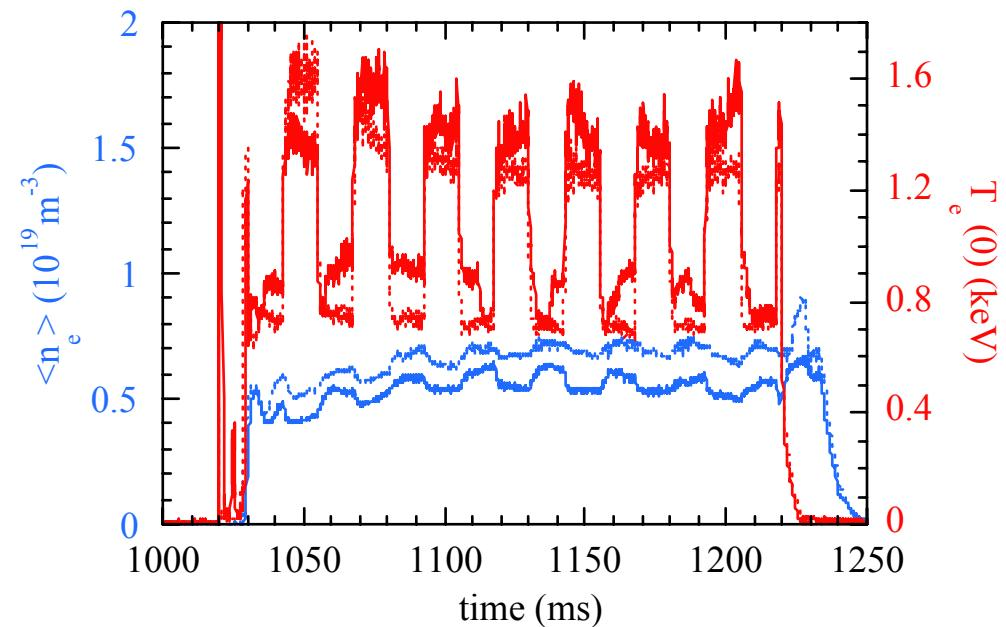
Magnetic configuration close to  $3/2$ . 300 kECH power modulation is enough to trigger eITB.
