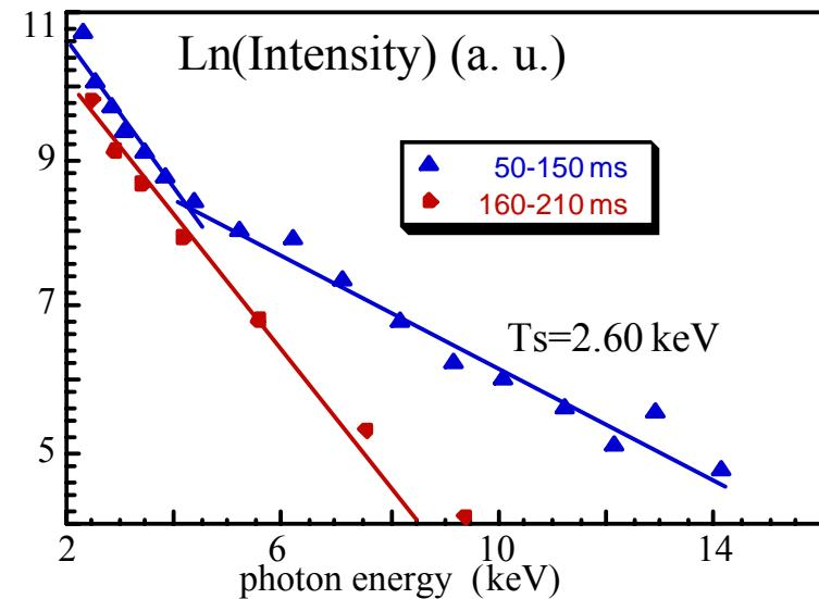
Temperature and density profiles, SXR spectra (100\_44\_64. Vacuum  $\iota(0)/2\pi=1.51$ ) with (blue) and without (red) eITBs.
