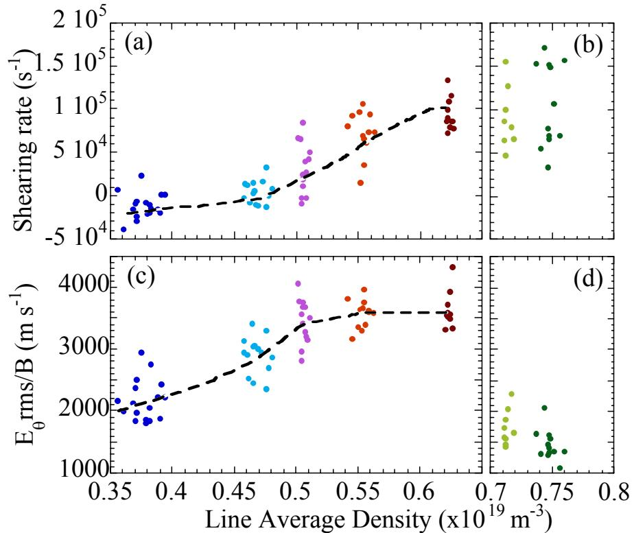
*Shearing rate vs. line density without (a) and with (b) polarised electrode and their corresponding turbulence levels (c,d).*
