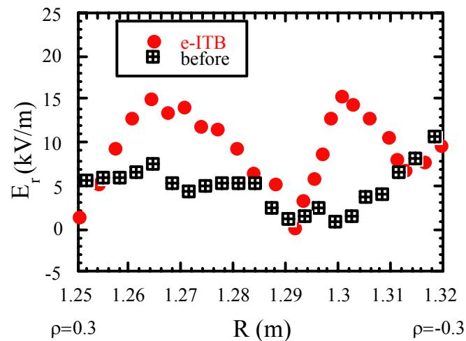
Te profile is steeper, plasma potential is more positive, (strong electric field appears, and central density falls).
