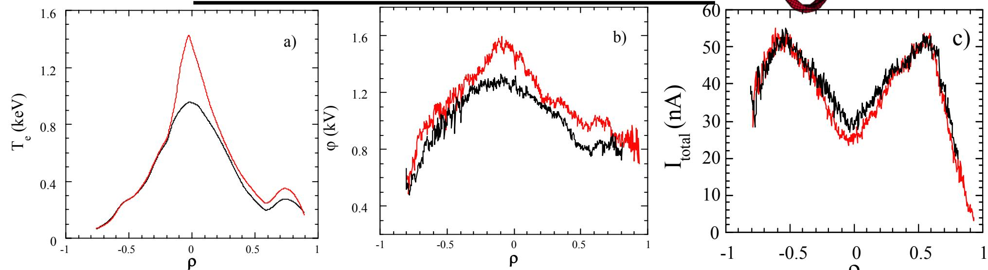
Te profile, plasma potential and beam intensity (proportional to density) with (red) and without (black) eITB
