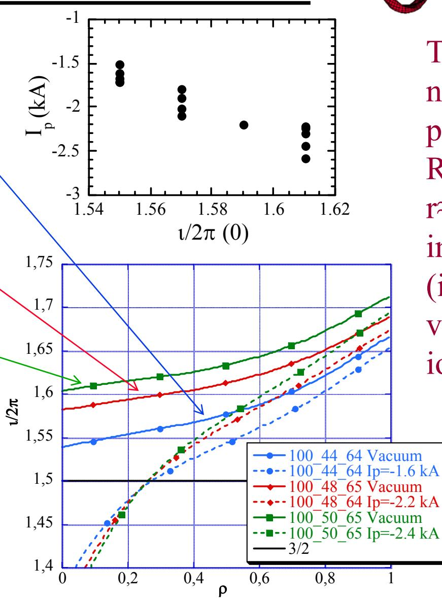
The Current needed to position the Rational at  $r \approx 0.2 - 0.3$  increases (in absolute value) with iota.
