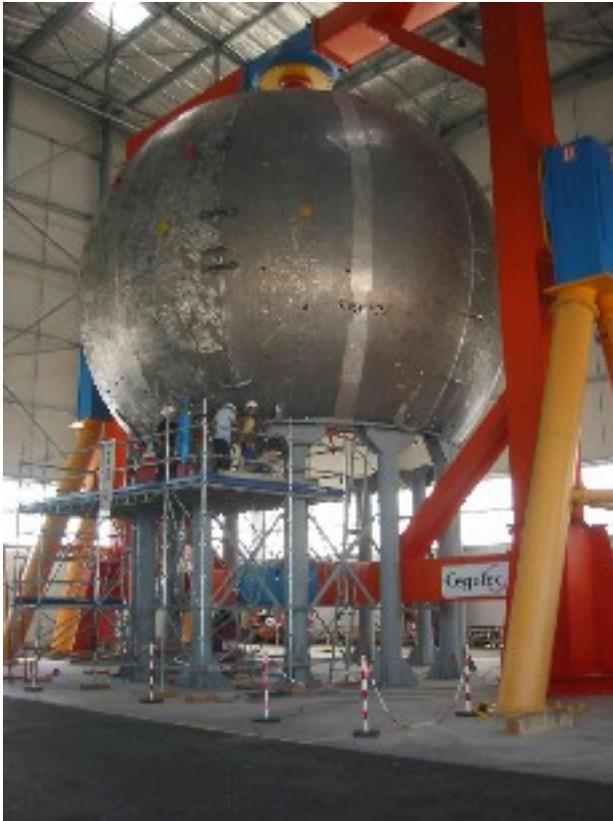
Target chamber (10m diameter)
