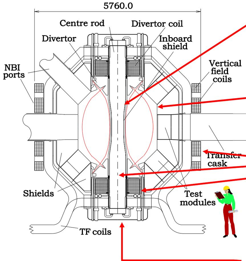
Tight aspect ratio means few neutrons absorbed on inner wall
