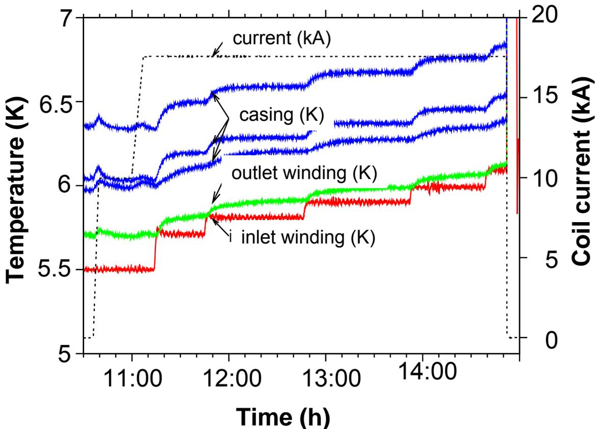
**Temperature and current signals during current quench test.**
