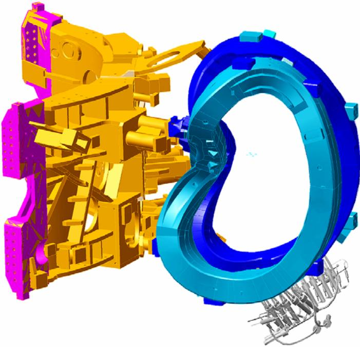
Connection is screwed using ~ 400 mm long rods in the form of a matrix of screws (up to 3x3)
