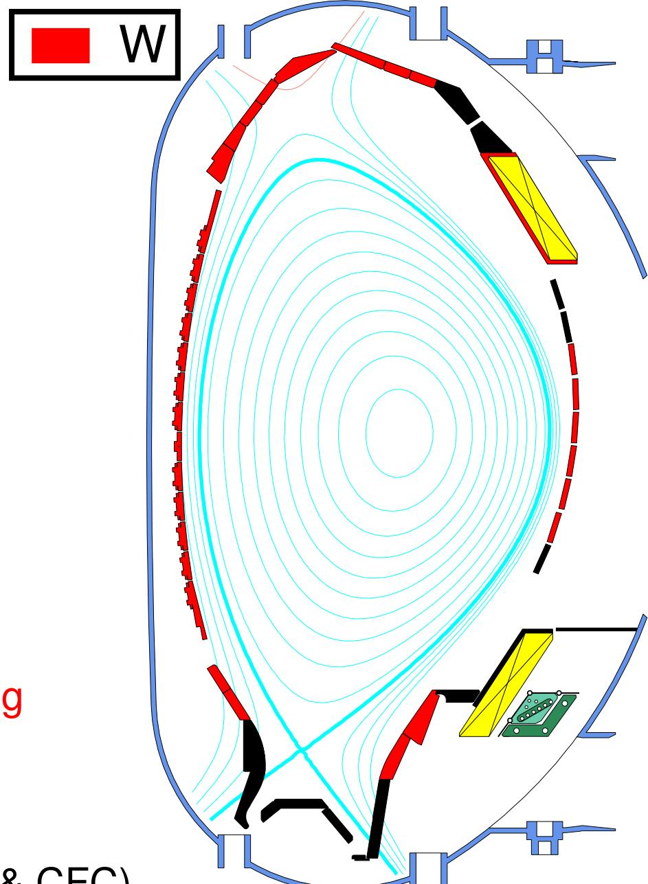
Step by step increase of W-coated plasma facing components (since 1999) towards a full W device
