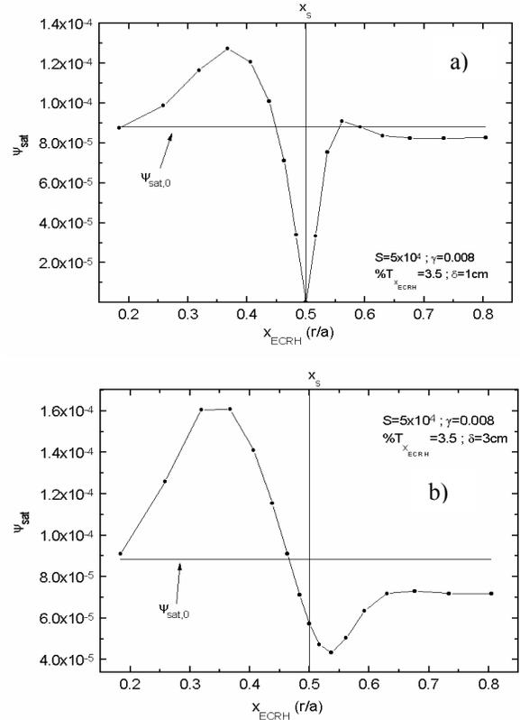
Fig. 7.6 - Normalised magnitude of reconnected (2,1) flux  $\Psi_s$  vs radial ECRH deposition: (a) for a deposition width of 1 cm, (b) for a deposition width of 3 cm, and for a  $q_0=1.5$  and  $q_a=3.5$  parabolic  $q$ -profile FTU-type (low viscosity  $\gamma$ ) discharge, calculated by a full non-linear tearing mode code in large  $R/a$  approximation.
