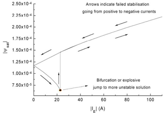
Fig. 7.2 - Normalised magnitude of reconnected ( $m=2, n=1$ ) flux  $|\psi_s|$  vs magnitude of external control current  $|I_E|$  for a  $q_0=1.2$  and  $q_a=4.2$  parabolic  $q$ -profile FTU-type discharge, calculated by a full non-linear tearing mode code in large  $R/a$  approximation
