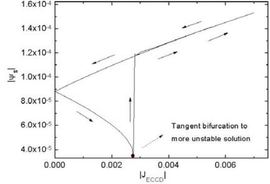
in Figs. 7.6a and 7.6b where the saturated Fig. 7.5 - Normalised magnitude of reconnected (2,1) flux  $|\Psi_s|$  vs magnitude of driven current  $|J_{ECCD}|$  for a  $q_0=1.5$  and  $q_a=3.5$  parabolic  $q$ -profile FTU-type discharge, calculated by a full non-linear tearing mode code in large  $R/a$  approximation.
