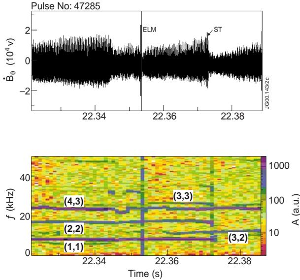
Fig. 7.1 – a) Magnetic signal and, b) Spectrogram showing the frequency and amplitude of modes observed around a sawtooth crash. It shows the sawtooth precursor (1,1) and its harmonics (2,2) and (3,3), a (4,3) mode unaffected by the sawtooth crash and the onset of a (3,2) mode observed above the noise level at 15 ms before the sawtooth crash.
