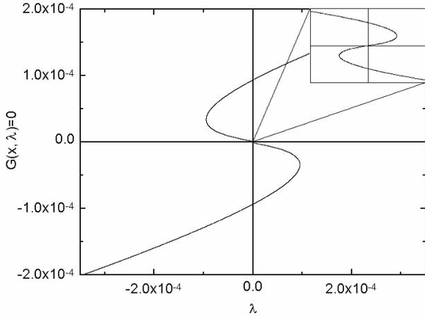
Fig. 7.3 - Equilibrium manifold  $G(X=\psi_s, \lambda \propto I_E)=0$  vs the control variable  $\lambda$  for “neoclassical” tearing mode model. The tangent bifurcation points and the local generic structure are apparent in the insert.
