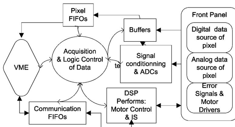
Figure 12.2 – Block diagram of the control and data acquisition module
