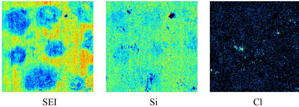
Figure 12.6 – Nuclear microprobe images from an uncoated SiC sample after the annealing conditions referred in the text. The images were obtained from a  $2640 \times 2640 \mu\text{m}^2$  scan, and the secondary electron image (SEI) clearly reveals the spots where the Be pebbles were in contact with the SiC material. Also shown are the Si and Cl maps.
