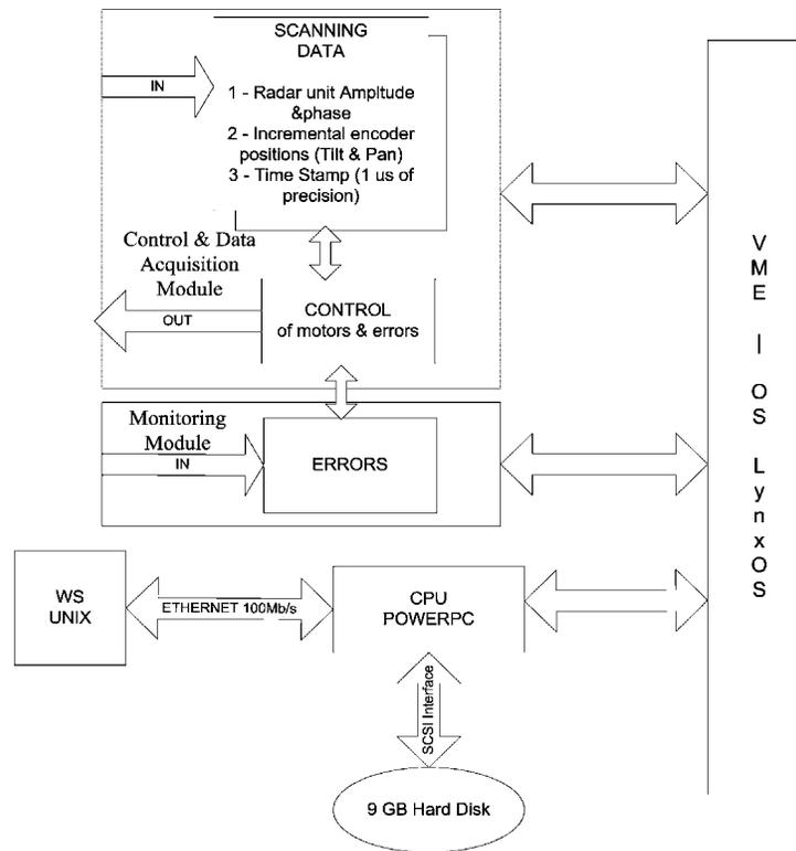
Figure 12.1 – Block diagram of CADAS
