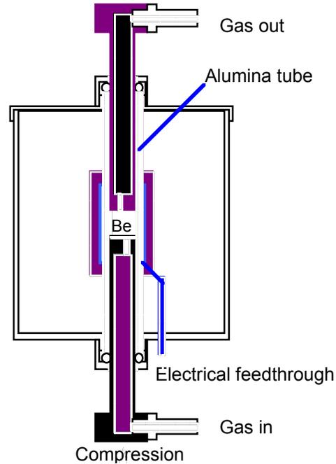
Figure 12.3 - Experimental set-up for the resistivity measurements with flowing gas.
