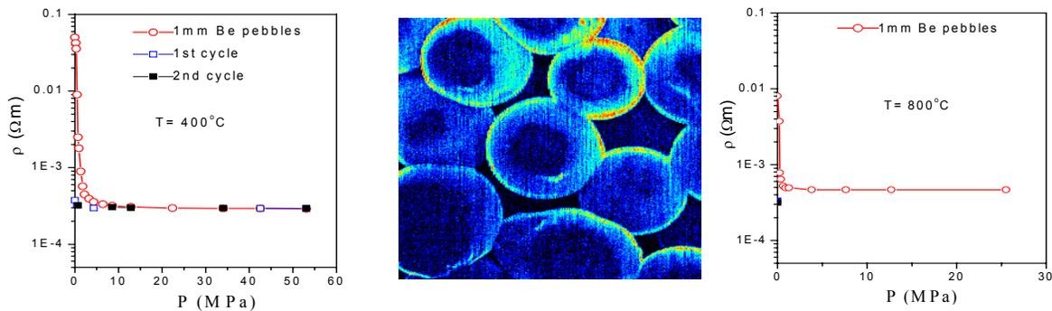
Figure 12.4 - Secondary electron image of a Be pebble annealed at 800°C and resistivity of the pebble bed at different temperatures as a function of the applied load.
