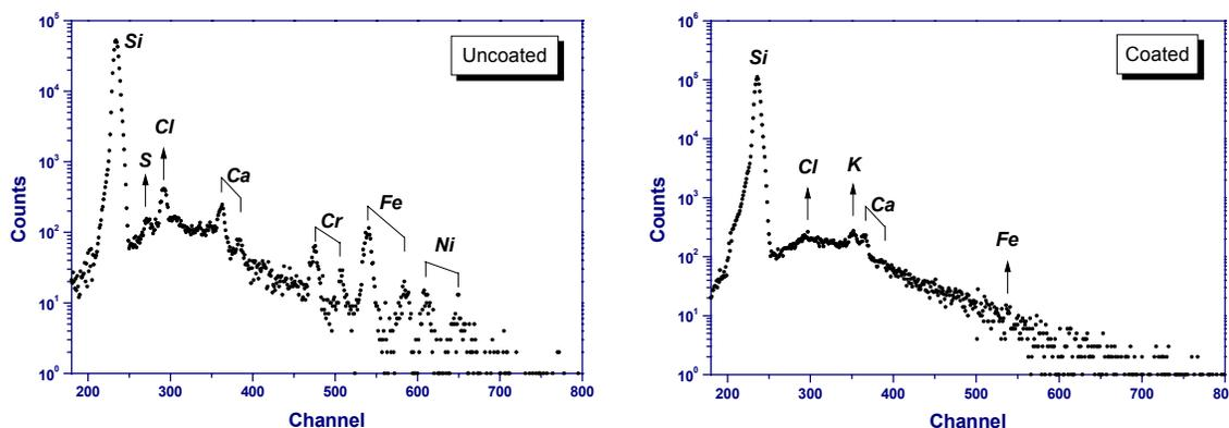
Figure 12.5 -  $\mu$ PIXE spectra of virgin uncoated (left) and virgin coated (right) samples showing the main contaminants. The spectra were obtained during a beam scan of 2640\*2640µm.
