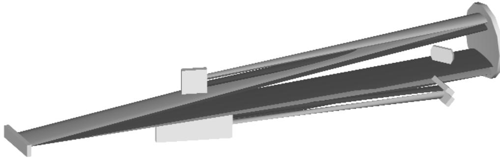
Figure 11.1 – Schematic of the new broadband grating stretcher
