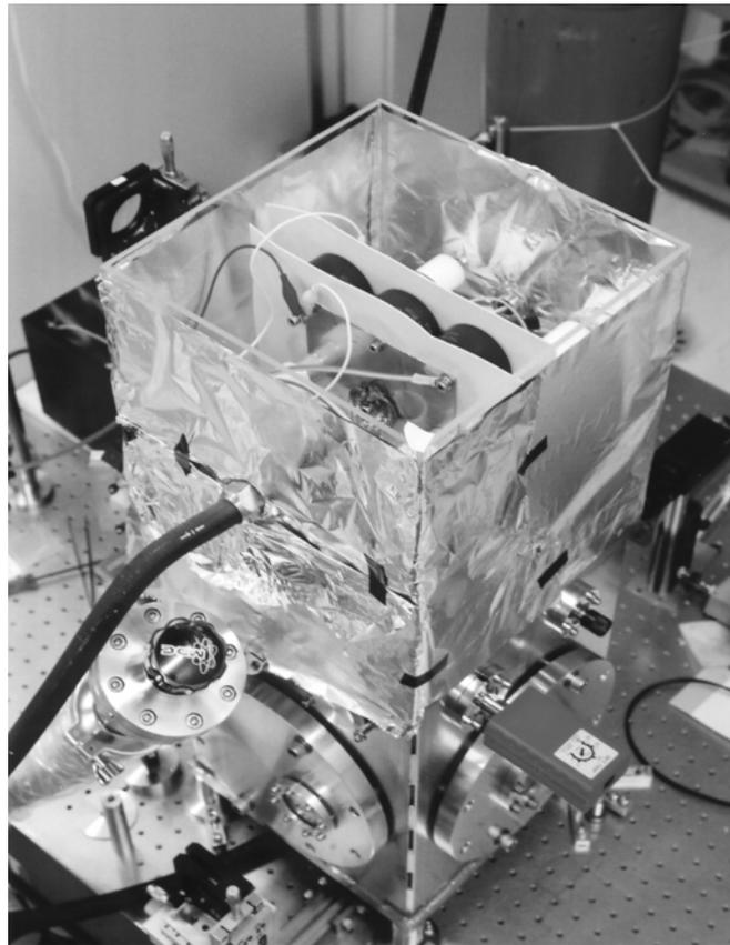
Fig. 11. 4 – Rendering of the vacuum chamber and insulated electrode mounts for the channeling scheme by laser-triggered HV
