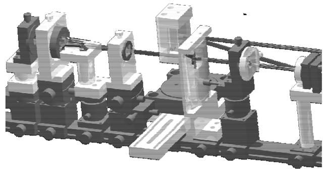
Figure 11.2 – Schematic of second-order single-shot autocorrelator
