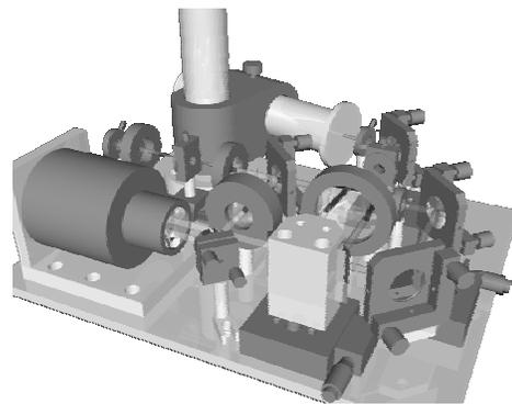
Figure 11.3 – Schematic of third-order scanning autocorrelator
