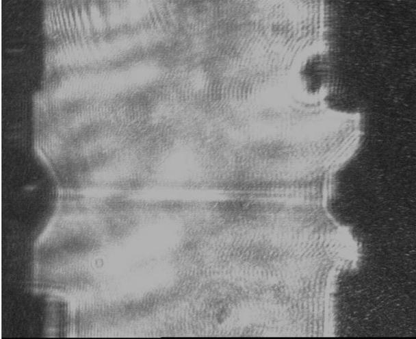
*Fig. 11.5 – Shadowgraphy of the first channel produced by the laser-triggered high voltage discharge channelling scheme*
