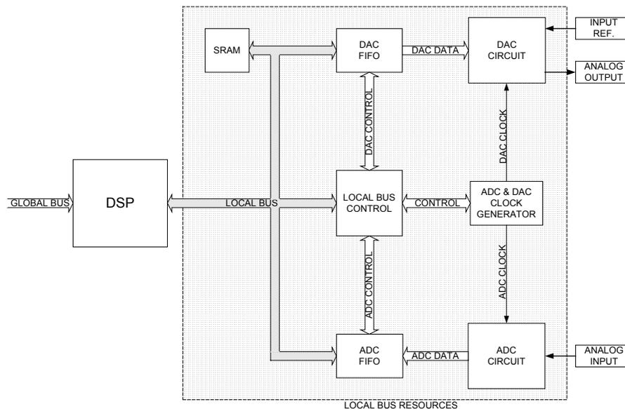
Figure 10.2 – Architecture of each acquisition, processing and control channel
