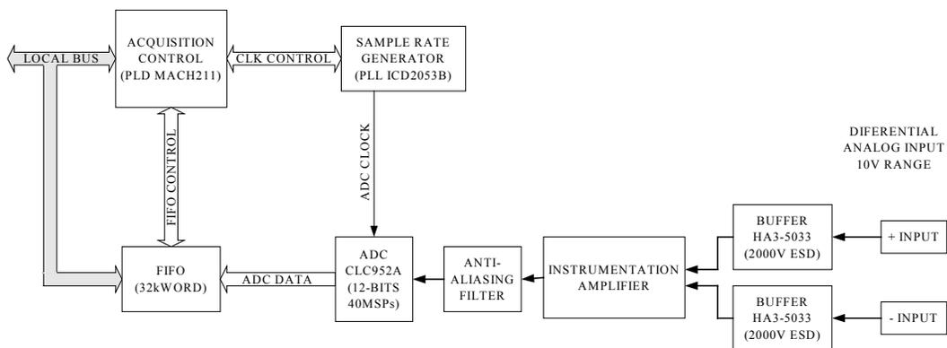
Figure 10.3 – Data acquisition architecture
