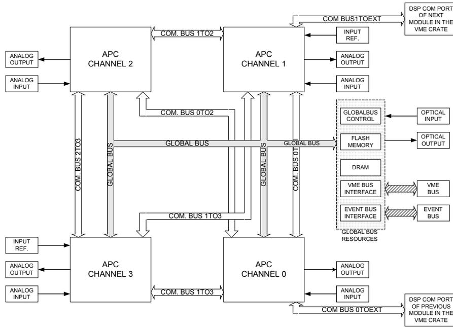
Figure 10.1 – Architecture of the intelligent module
