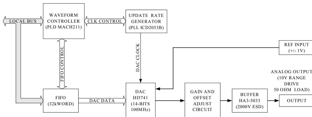
Figure 10.4 – Control and waveform generator architecture
