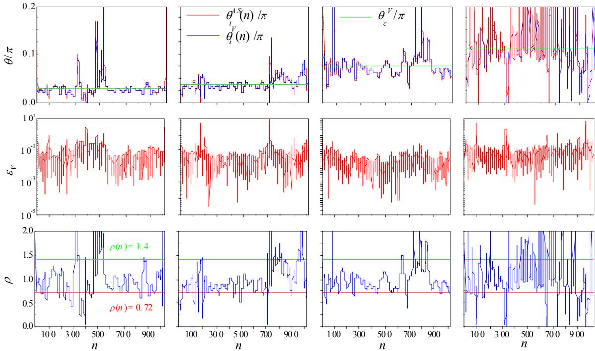
Figure 10.6 - Carrier frequencies, instantaneous frequencies, and relative errors for typical data from four O-mode reflectometry channels calculated using the analytic signal and the variational method.
