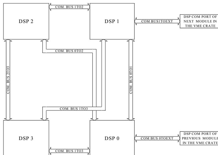
Figure 10.5 – DSP inter-communications buses structure
