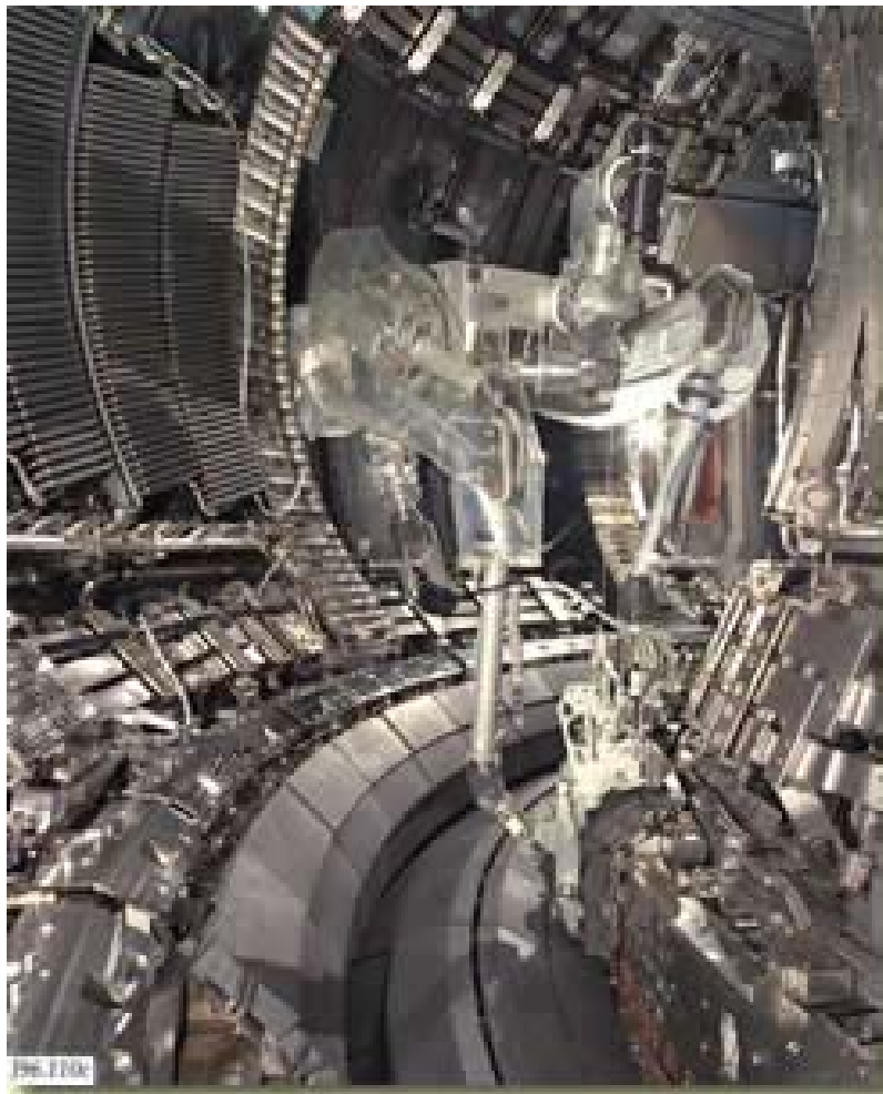
Figure 1.2 – Manipulator installing the tiles of the JET Mark II divertor
