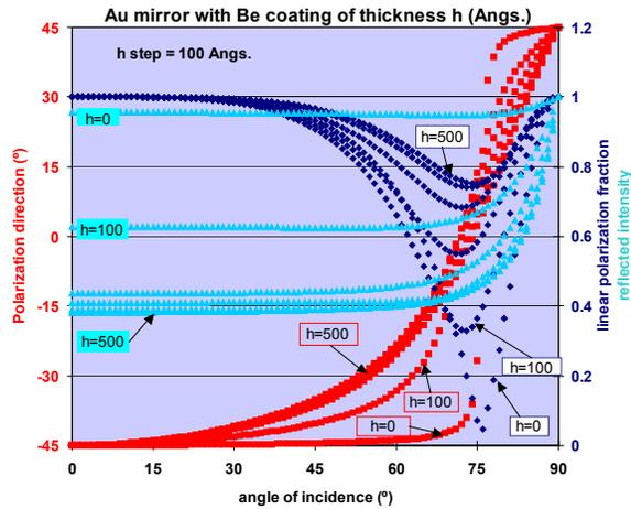
Figure 8.2 – The graph shows how Be coating ( $h$ ) affects the polarization state of light (linear polarization fraction), direction and total reflected intensity.
