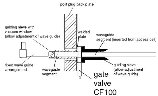
Figure 8.10 – a) Rearrangement of diagnostics in the port plug and b) example of introduction of local safety and confinement rules for wave guides compatible with automatic coupling (work in progress).
