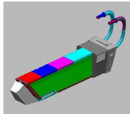
Figure 8.11 - Actual water feeding pipes can have an interference with diagnostic components.
