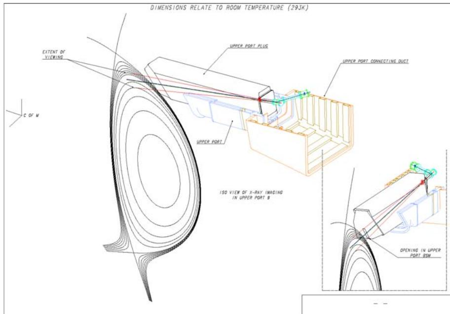
Figure 8.8 - Imaging X-ray system for uport9
