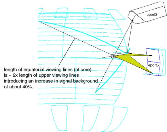
Figure 8.6 – Edge system at uport4 is replaced by pure toroidal edge system at eport3 (upper system). An edge to core system is introduced at eport3 (lower system) allowing the retrieval of edge poloidal velocity. The eport3 systems will enable MSE measurements of very high spatial resolution with retrieval of magnetic field pitch angle and  $E_r$ .
