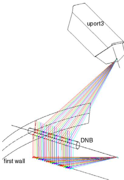
Figure 8.5 – Core CXRS viewing lines arrangement
