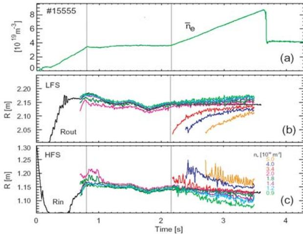
Figure 8.13 - Temporal evolution of: (a) line average density from interferometry; (b) position of the magnetic separatrix at the low field side ( $R_{out}$ ) inferred from the magnetic diagnostics and position of layers with constant density from reflectometry; (c) position of the magnetic separatrix at the high field side ( $R_{in}$ ) and position of layers with constant density from reflectometry.
