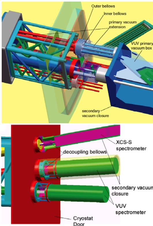
Figure 8.9 – Old arrangement at a) eport11 and b) uport10. Secondary enclosures connected to cryostat door are to be removed and its function implemented in a ‘localized per diagnostic’ way implying rearrangement of diagnostic distribution.
