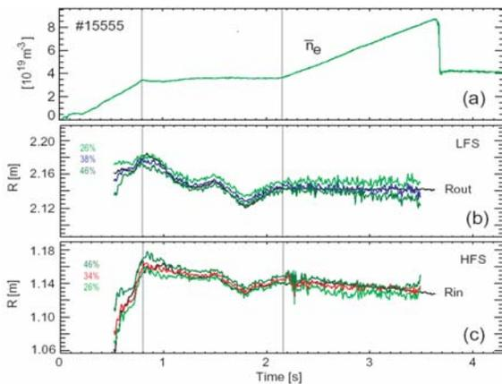
Figure 8.14 - Plasma position from reflectometry tracking density layers related to the line average density by different percentages. The best match between the data from reflectometry and from the magnetics is obtained for a 38% scaling on the LFS (blue curve) and for 34% on the HFS (red curve).
