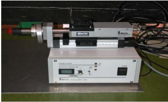
Figure 7.2 - Photo of the SDD detector plus the electronic cooling system and its monitor.
