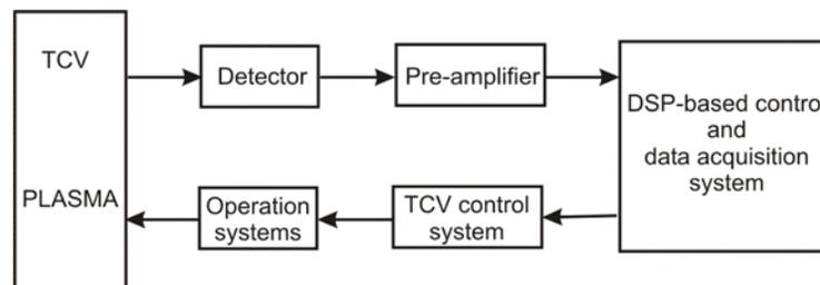
Figure 7.1 – Block diagram of the vertical PHA diagnostic
