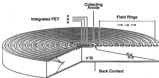
Figure 7.3 - Schematics of the SDD wafer
