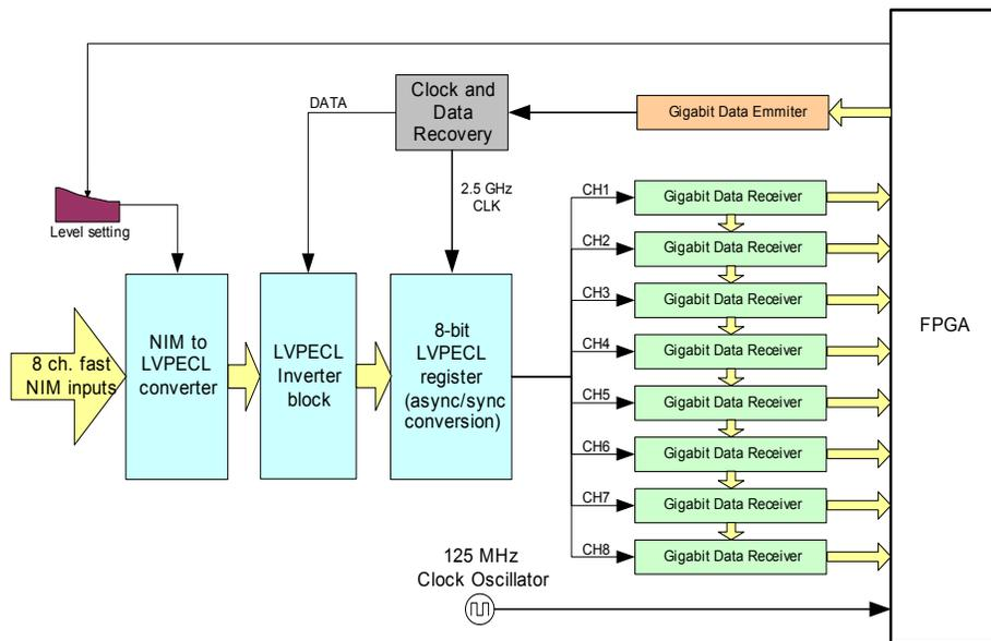
Figure 10.2 – The 2.5 GHz PECL time to digital converter
