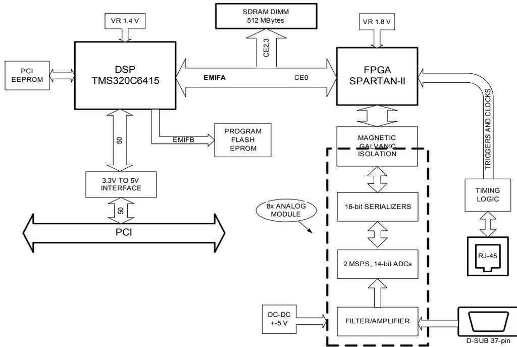
Figure 10.1 – The PCI-TR-256 module architecture
