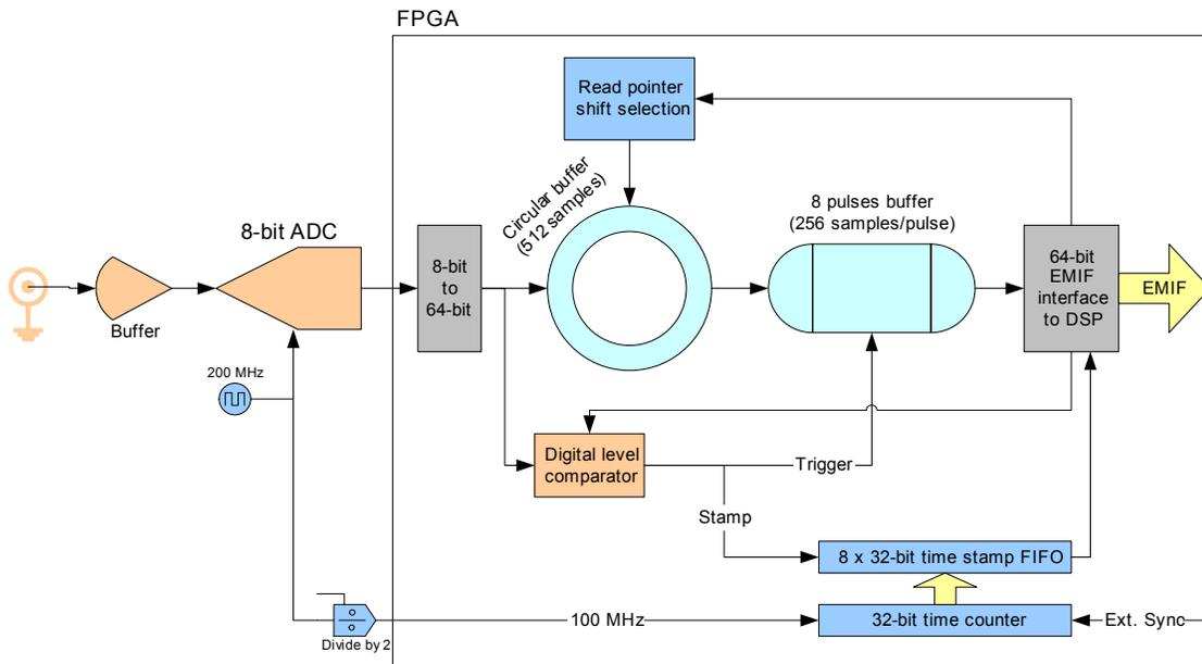
Figure 10.3 - Control and data flow through the FPGA for one ADC channel
