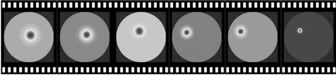
*Figure 10.3 – Frames taken from a plasma current position movie, were only six of 80 are presented.*
