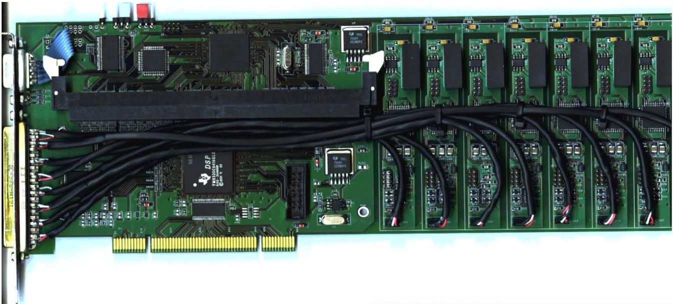
Figure 10.1 - Eight channels galvanic isolated transient recorder module
