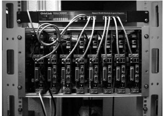
Figure 10.2 - Front view of the Orionte cluster.
