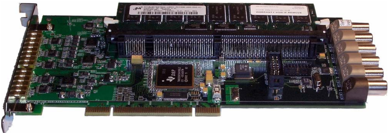
Figure 3.34 - Time digitizer module.
