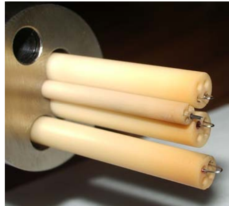
Figure 2.4 - The ISTTOK probe system, consisting of three emissive probes and one cold probe.
