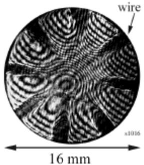
Fig3. End-on laser interferometry
