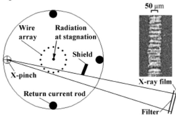
Fig 1. Schematic of the Xpinch backlighter
