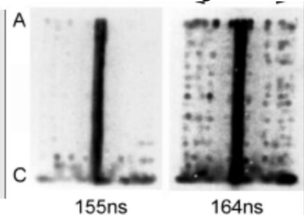
Fig. 5. Gated X-ray image of precursor and global m=0 mode
