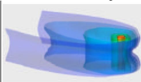
Fig. 4. Density surfaces from a 3D MHD simulation of a wire in an array during the breaking phase.
