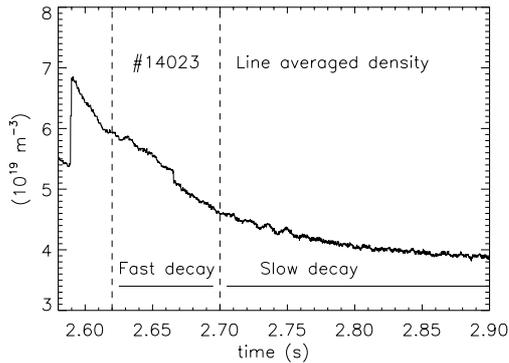
Figure 2: *Density decay after injection of last pellet*
