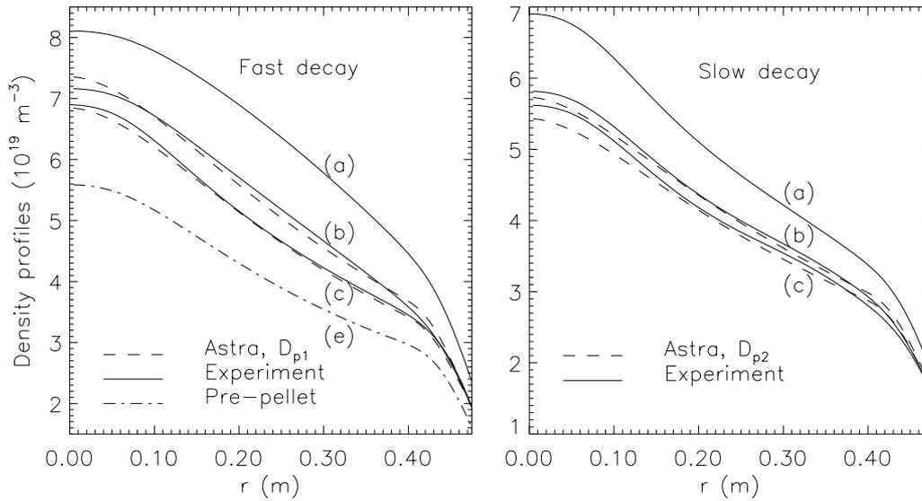
Figure 3: Comparison between calculated and experimental density profiles
