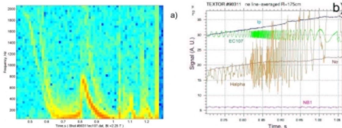
FIG. 4. Mode dynamic frequency behaviour during a ramp up phase of the discharge around 0.82 s ( $I=320$  kA,  $n_e=2.1\cdot 10^{19}$  m $^{-3}$ ). The mode frequency is jumping from 100 to 800 Hz in less than 100 ms (Fig. 4a). Figure 4b shows an enhancement of  $H_\alpha$  signal during the frequency change. For this shot, the  $m=2$  mode is coupled to the  $m=1$  mode.
