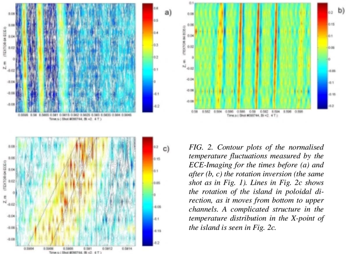
FIG. 2. Contour plots of the normalised temperature fluctuations measured by the ECE-Imaging for the times before (a) and after (b, c) the rotation inversion (the same shot as in Fig. 1). Lines in Fig. 2c shows the rotation of the island in poloidal direction, as it moves from bottom to upper channels. A complicated structure in the temperature distribution in the X-point of the island is seen in Fig. 2c.
