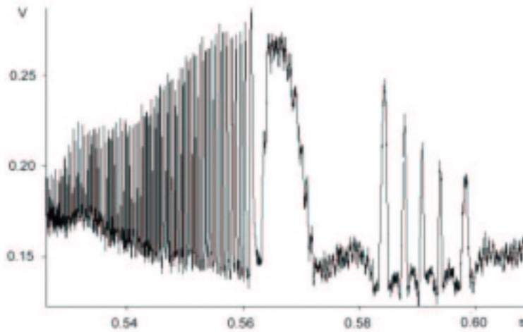
FIG. 1. A large  $m=2$  mode monitored by the ECE-Imaging system (raw data). The toroidal rotation inversion due to co-NB injection occurred at  $\sim 0.565$  s. X-point of the island is clearly seen as series of voltage peaks. Magnetic field  $B = 2.4$  T.
