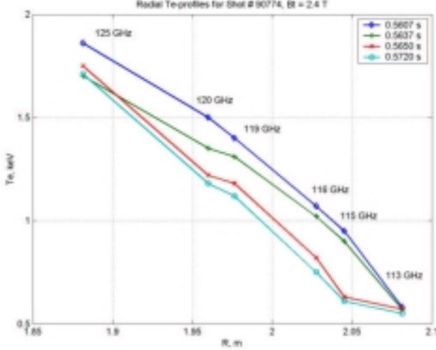
FIG. 3. Radial temperature evolution throughout the  $m/n=2/1$  island. The profile at 0.5607 s shows the temperature distribution at the X-point, and profiles at 0.565 s and 0.572 s in the vicinity of the O-point. Temperature flattening (compare to the X-point) inside the island is clearly seen at  $R = 2.04-2.07$  m. Absolute values for temperature gradients are calculated to be 4-6 keV/m at the X-point.
