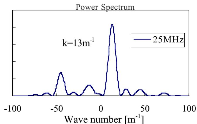
Fig. 1 The  $k_\phi$  spectrum measured in front of the TST-2 combline antenna by a magnetic probe, in the absence of plasma. The peak toroidal wavenumber of  $k_\phi = 13 \text{ m}^{-1}$  corresponds to a toroidal mode number of  $n = 7.4$ .
