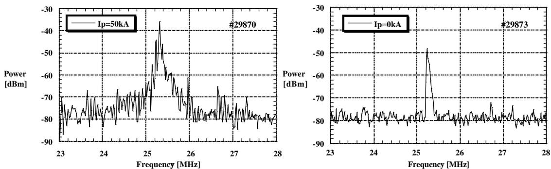
Fig. 2 Comparison of the frequency spectrum with (left) and without (right) plasma. The HHFW field was detected by a probe located on the low field side, approximately  $30^\circ$  away in the toroidal direction from one end of the antenna.
