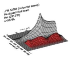
Fig.4: Beam emission profile showing the Doppler-shifted emission (right, red) and the unshifted emission (left) for a 6s doped 74 kV beam.
