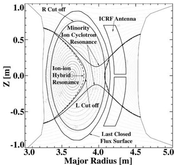
*Fig.1 The resonance and cutoff diagram in the optimum heating regime. The antenna is located in the toroidal section where plasma cross section is vertically elongated. In front of the antenna, there is a region where magnetic field has weak non-uniformity.*
