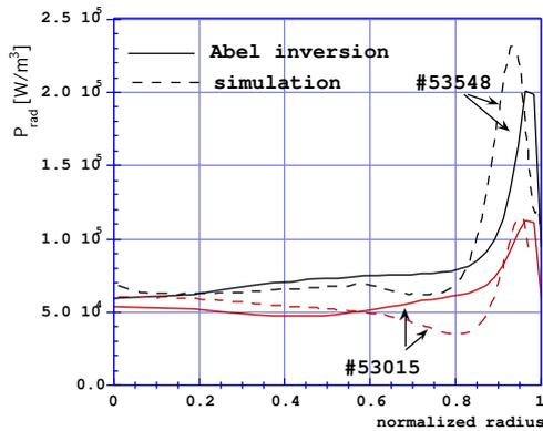
Fig. 4 : Radial profile of the radiated power density during the quasi-stationary high confinement phase for shots #53015 ( $t=61$  s) and #53548 ( $t=62$  s)
