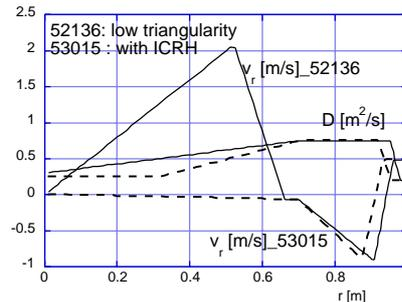
Fig.2 : Diffusion coefficient and pinch velocity for shots #52136 and #53015 at  $t=60\text{s}$
