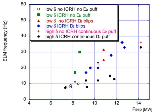
Fig. 6: ELMs frequency vs the power at the separatrix, calculated during the stationary phase as  $P_{tot} - P_{rad}$
