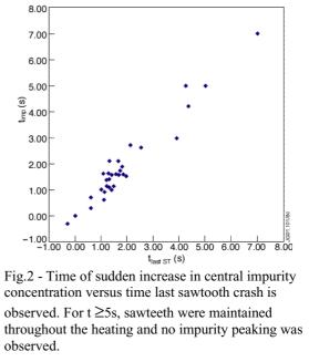
the ELM-free periods, or following large type I ELMs was evaluated as a contributor to the confinement degradation. Bolometer data analysis indicated that central impurity accumulation occurred in a variety of ELM regimes, including Type III ELMs. Soft-X-ray emission indicated that following Type I ELMs the impurity density increases in the outer region of the plasma, typically within 20-30 cm from the edge.
