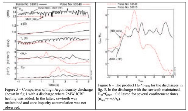
V Conclusions - Maintaining sawteeth using ICRF heating resulted in quasiady state, high performance plasmas with high Ar densities. Values  $\delta f_{97} * f_{GWD} \sim 0.8$ , previously only lasting  $<1 \tau_E$  at high Ar injetion rates, were maintained for the duration of the heating( $\Delta t \sim 9 \tau_E$ ). We conclude sawtooth plays an important role in preventing impurity accumulation.
