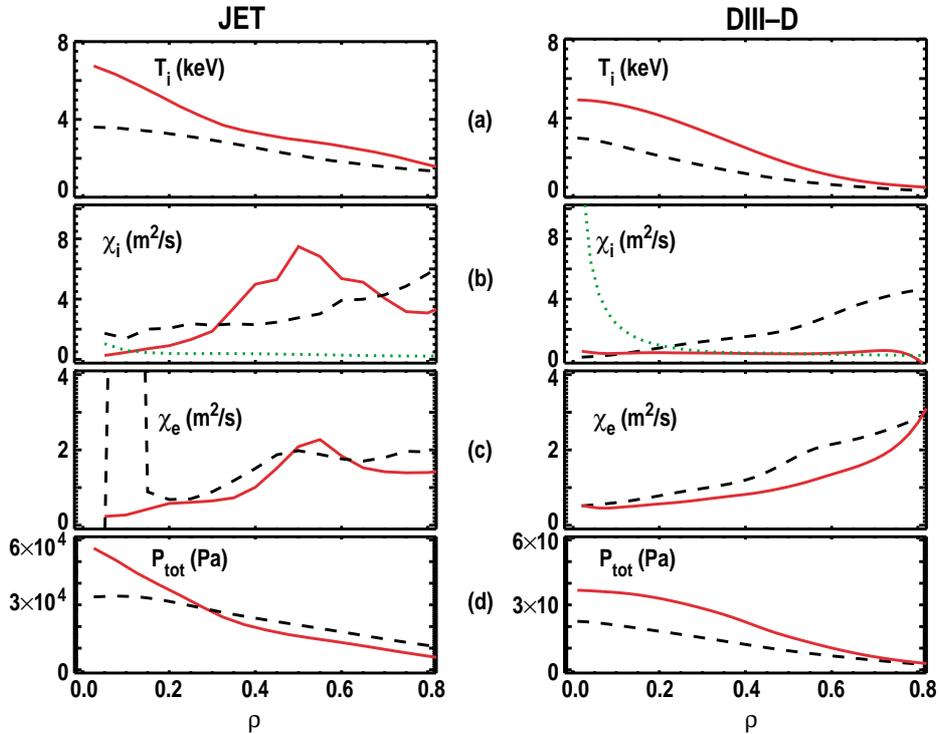
Fig. 2. Profiles of (a)  $T_i$ , (b)  $\chi_i$ , (c)  $\chi_e$ , and (d) plasma thermal pressure for both JET (left panels) and DIII-D (right panels) at 44.8 s (JET) and 1.16 s (DIII-D). Ion neoclassical diffusivity is shown as a dotted line (b). Reference discharges (no neon) are shown as dashed lines. Discharges are the same as those in Fig. 1.
