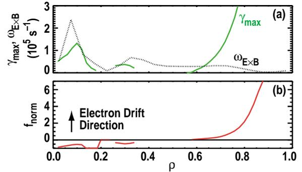
Fig. 4. Maximum growth rate and calculated  $\mathbf{E} \times \mathbf{B}$  shearing rate for JET pulse #53154 with neon seeding (a). Normalized frequency (b) indicates the  $\gamma_{\max}$  is in the ion diamagnetic drift direction for  $\rho < 0.4$  and the electron diamagnetic drift direction for  $\rho > 0.6$ .
