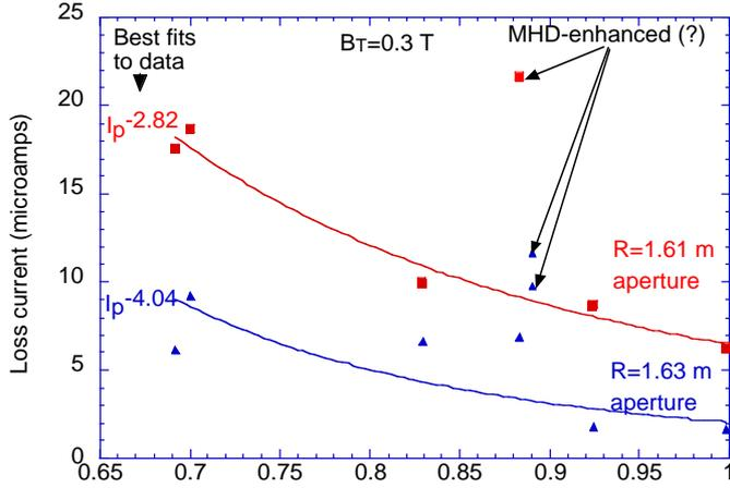
Figure 2: Measured beam ion loss currents at the NSTX midplane as a function of plasma current. Shown also are power law fits to
