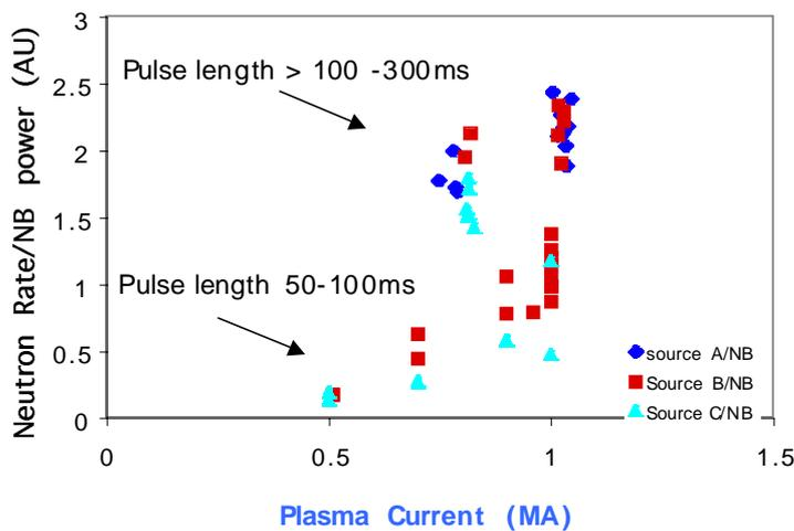
loss and collisional effects, for the several shots that have been analyzed. Similarly, the neutron decay time after NB turn off usually matches that computed from the collisional slowing down of the NB ions, suggesting no large anomalous losses.
