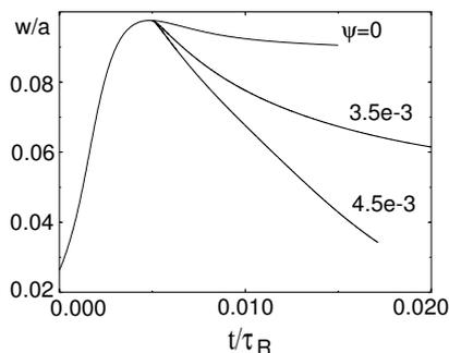
Fig.5 The time evolution of the normalized 3/2 island width with  $\psi=0$ , 0.0035 and 0.0045, respectively.
