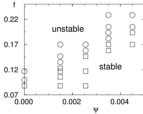
Fig.4 The required  $\psi$  for stabilizing the 3/2 mode. The squares (circles) denote the stable (unstable) cases.
