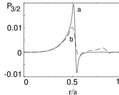
Fig.6 The 3/2 pressure perturbations without (a) and with the 2/1 mode and their couplings (b) from XTOR.
