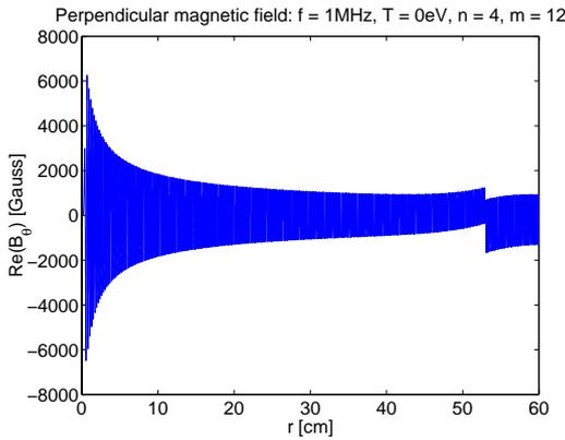
Fig. 3. Radial profile of the perpendicular magnetic field  $\text{Re}(B_\vartheta)$  after solving for the boundary conditions at the antenna location,  $r=53$  cm. The discontinuous behavior of  $B_\vartheta$  and  $B_z$  corresponds to the prescribed (Fourier decomposed) antenna currents.
