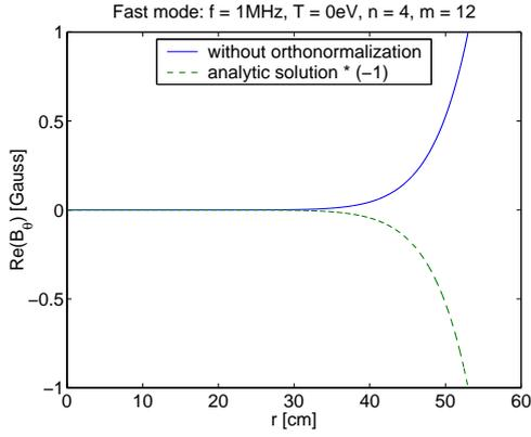
Fig. 1. The fast mode ( $k_{r,f} \approx i \frac{m}{r} \text{cm}^{-1}$ ) obtained numerically (solid line) and the analytical solution (dashed line) drawn with negative sign for comparison.
