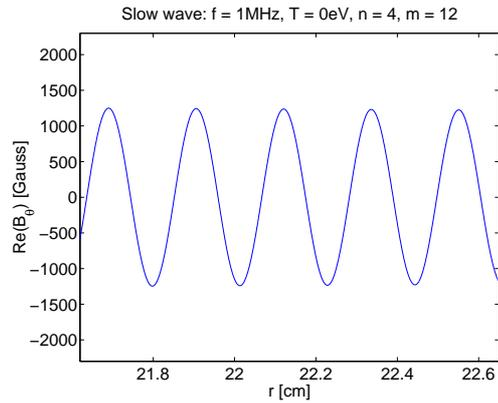
Fig. 4. Using the orthonormalization algorithm one can actually resolve the slow mode behavior with wave length  $\lambda_{r,s} \approx 0.22 \text{cm}$  (detail of Figure 3).
