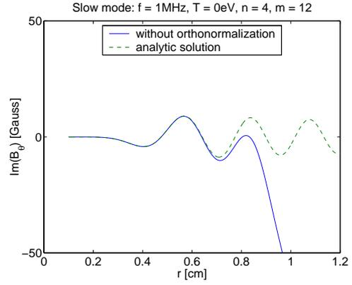
Fig. 2. The slow mode evolution obtained numerically without reorthonormalization (solid line) and the analytical solution (dashed line). After a couple of oscillations the numerical solution starts to grow similar to the fast mode due to finite numerical precision.
