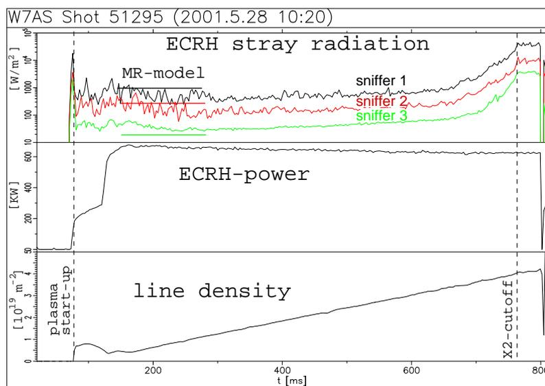
Fig. 3: Development of the stray radiation in a discharge, when the plasma density was risen up to above the X2-cutoff. The horizontal bars are results of the MR-model using an average plasma absorption of 50% (X2-mode and O2-mode) and a total stray radiation power of 2 kW.
