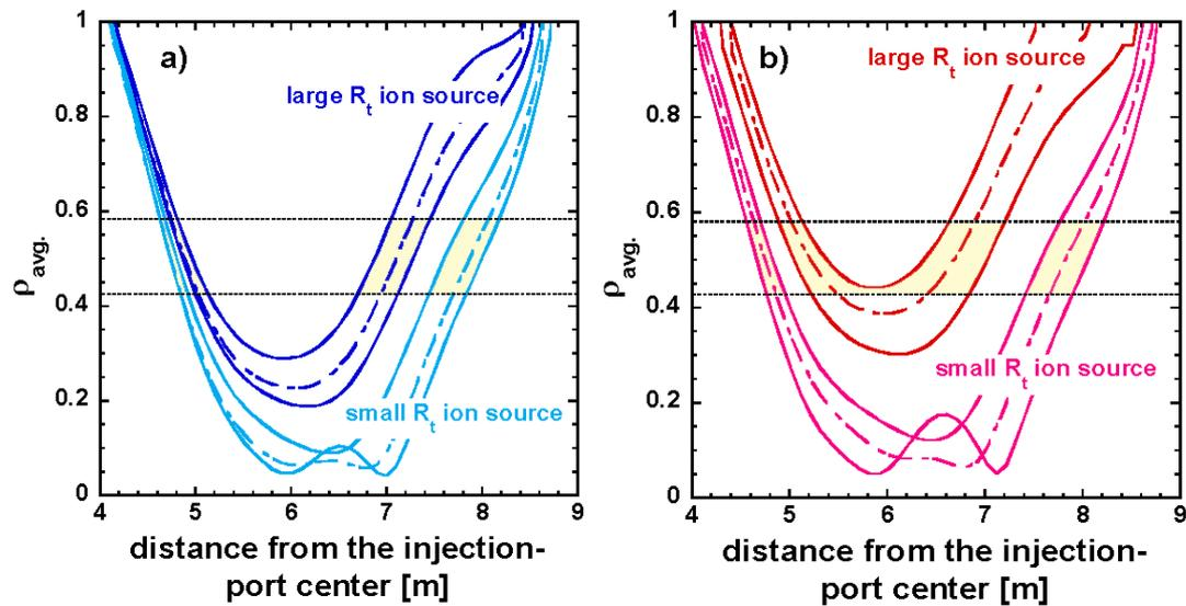
**Fig.4** The  $\rho_{avg}$ -distribution along NB flight paths for (a)co.-NB and (b) ctr.-NB injectors. The yellow regions show the ICRF interacting domains where the particle launched from the sight line of ion sources enters ICRF-resonance region, frequently.
