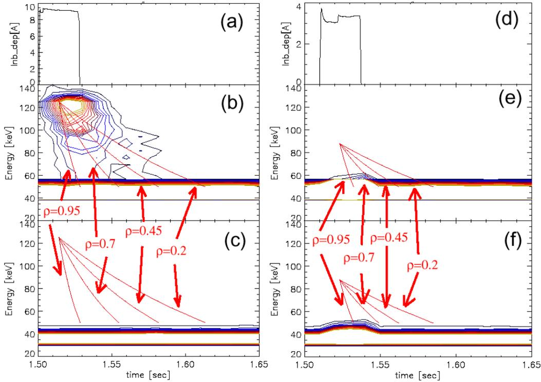
**Fig. 2** a) NB deposition current to plasmas, b) contour plot for tangential Si-FNA spectra and c) contour plot for perpendicular Si-FNA for co.-NB blip injection. (d),(e) and (f) are these for ctr.-NB blip injection. Red curves in contour plots show the slowing-down curves of NB-particles at various location of plasmas.
