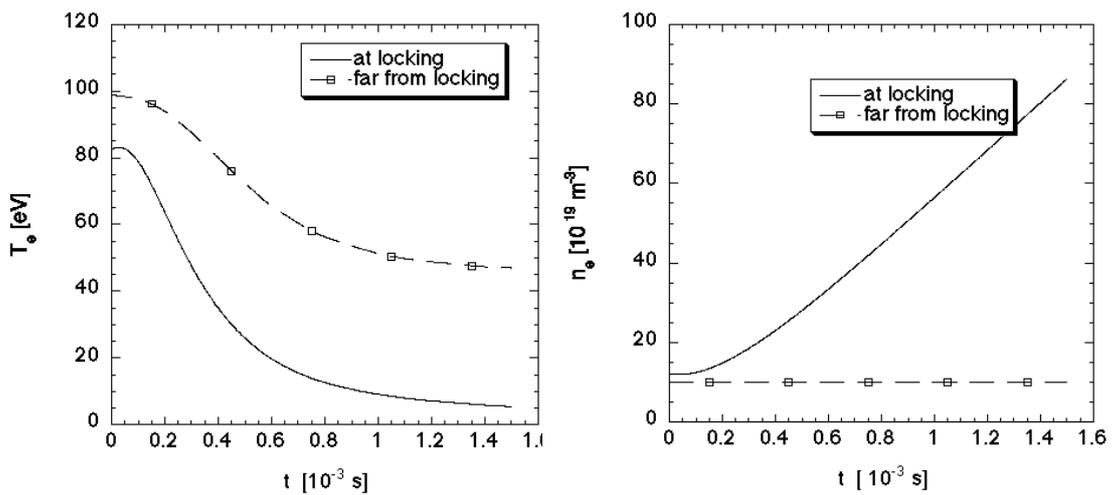
Fig.2 Time evolution of electron temperatures and densities in the region at locking and in the remaining plasma with the hydrogen influx at locking increasing in time  $\Gamma = 10^{23} - 10^{24} \text{ m}^{-2} \text{ s}^{-1}$
