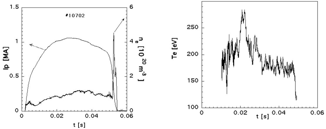
Fig.1 Time waveforms of  $I_p, n_e, T_e$ , during a RFX high current, fast terminated discharge
