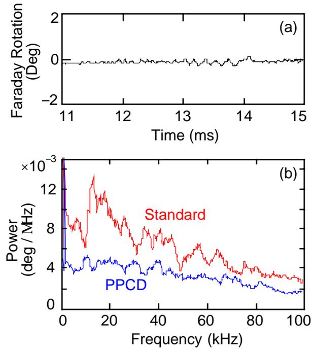
Fig. 3 (a) Faraday rotation angle showing fluctuation corresponding to internal  $m=1$  modes, and (b) frequency power spectra in PPCD and standard plasmas.
