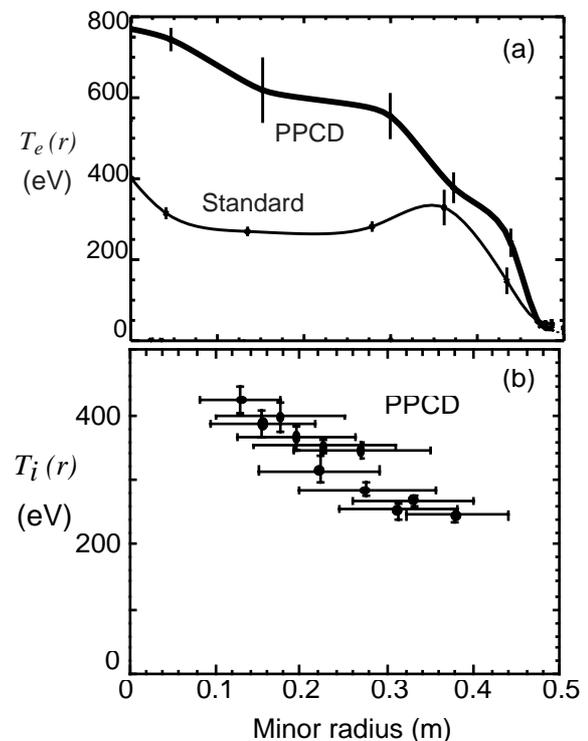
Fig. 4 (a) Electron and (b) majority ion temperature profiles.
