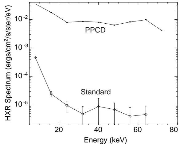
Fig. 2 Energy spectra of the HXR flux from PPCD and standard plasmas.
