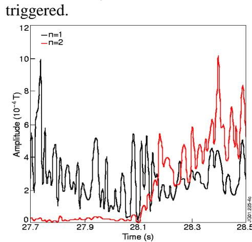
Figure 4: Amplitude of the  $n=1$  fishbone bursts and  $n=2$  NTM modes for the shot #52083
