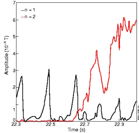
Figure 2: Amplitudes of the  $n=1$  sawtooth precursor and  $n=2$  NTM mode for the shot #51995
