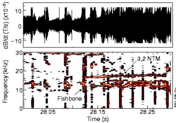
Figure 3: Induced Signal in a fast pickup coil from the shot #52083 and its correspondent spectrogram showing a NTM triggered in a discharge with frequent fishbones
