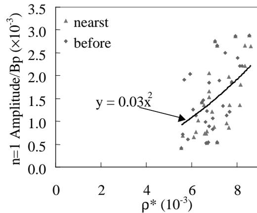
Figure 7:  $n=1, m=1$  amplitude normalised by  $\rho^*$
