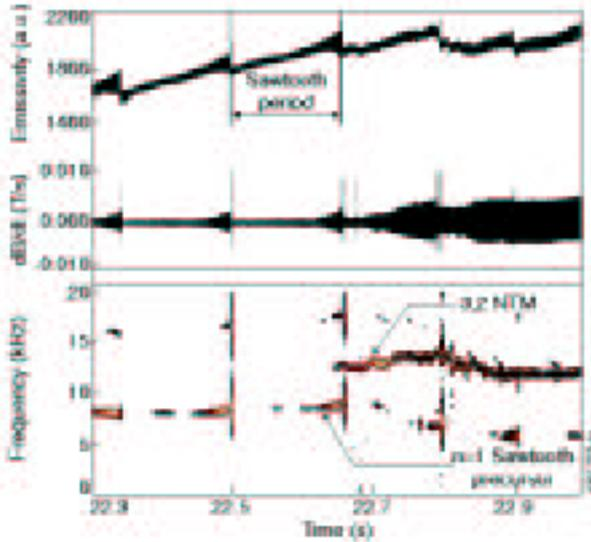
Figure 1: Signal from the Soft X-ray central emission, induced signal in a fast pickup coil from the shot #51995 and the correspondent spectrogram showing a (3,2) NTM triggered shortly before a sawtooth crash.
