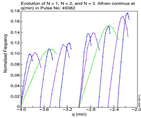
**Fig.7** Modelling of the Alfvén cascades of different toroidal mode numbers  $n=1$  (green),  $n=2$  (red) and  $n=3$  (blue) in #49382 with gradually decreasing  $q_{\min}$ .
