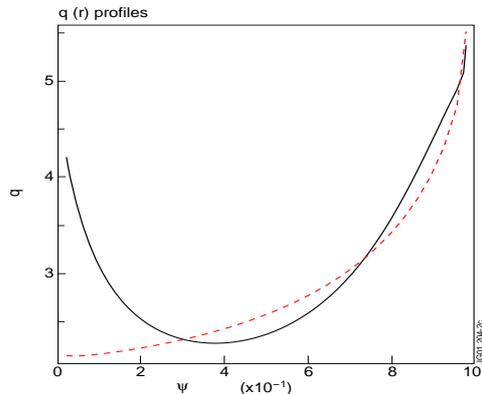
**Fig.2** Safety factor profiles  $q(r)$  reconstructed from EFIT. MSE was used for reversed shear case #49382.
