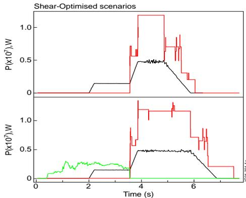
**Fig.1** Two OS discharges (pulses #49384 and #49382 with  $B_T=2.6$  T and  $I_P^{\max} = 2.2$  MA) with the only difference in 2.5 MW of LHCD
