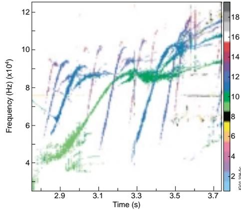
**Fig.5** Toroidal mode numbers of ACs shown in Figure 4
