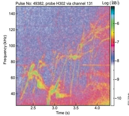
**Fig.4** Spectrogram of the magnetic perturbations in plasma with **non-monotonic**  $q(r)$ . Alfvén cascades are observed at frequencies below TAE frequency,  $f_{AC} \cong 30-100$  kHz  $<$   $f_{TAE}$ .
