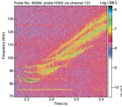
**Fig.3** Spectrogram of the magnetic perturbations,  $\delta B_p$  (Tesla), measured by Mirnov coils in plasma with **monotonic**  $q(r)$ . TAE modes are seen at frequencies  $f_{TAE} \cong 80-200$  kHz.
