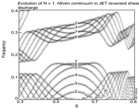
**Fig.6** CSCAS code: frequency  $\omega R_0 / V_A(0)$  of Alfvén continuum as a function of radius  $s = (\psi_P / \psi_P^{edge})^{1/2}$
