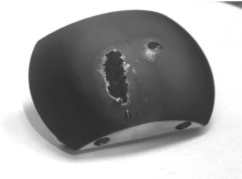
*Fig. 1 B<sub>4</sub>C coated limiter after the exposure to the plasma. Dimensions of test limiters: projected length 120 mm (toroidal direction), projected width 60 mm (poloidal direction), radius of curvature 140 mm, height 45 mm, area of the plasma facing surface 100 cm<sup>2</sup>. The lines of analyses were crossing the damaged areas.*
