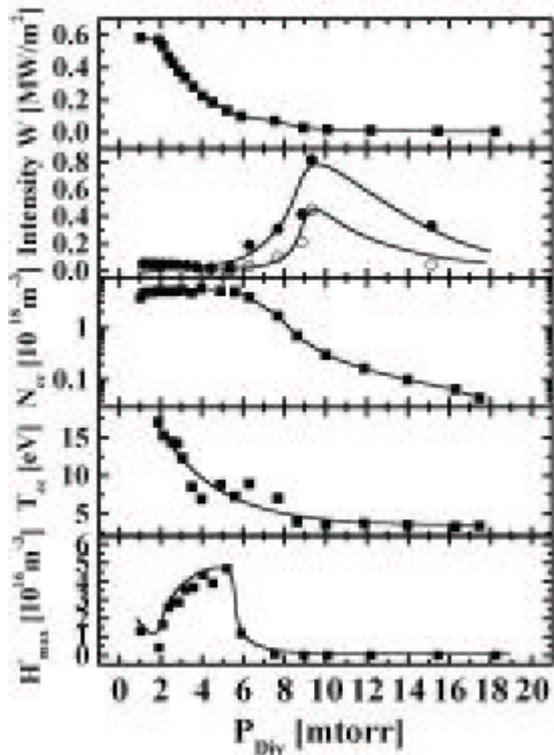
Fig.1 The dependence of W, the hydrogen and helium Balmer spectrum of visible light emission closed circle  $H_\gamma(2p-5d)/H_\alpha(2p-3d)$  and open circle  $He(2p-5d;T)/He(2p-3d;T)$ , the variations electron density  $N_{ec}$ , the electron temperature  $T_{ec}$  at the center of sheet plasma, and the maximum value to the y-direction profile of  $H_{max}$ , on hydrogen gas pressure.
